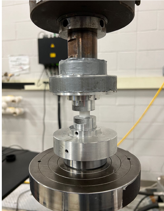
Fig. 8 Loading setup for quasi-static and intermediate rate experiments
