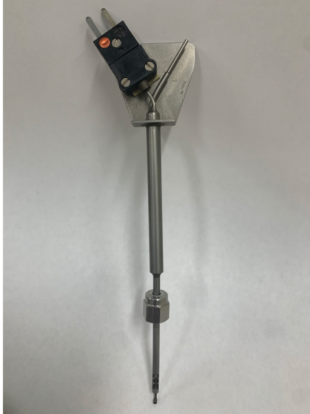
Figure 34. Current Kiel probe/ thermocouple combination.
