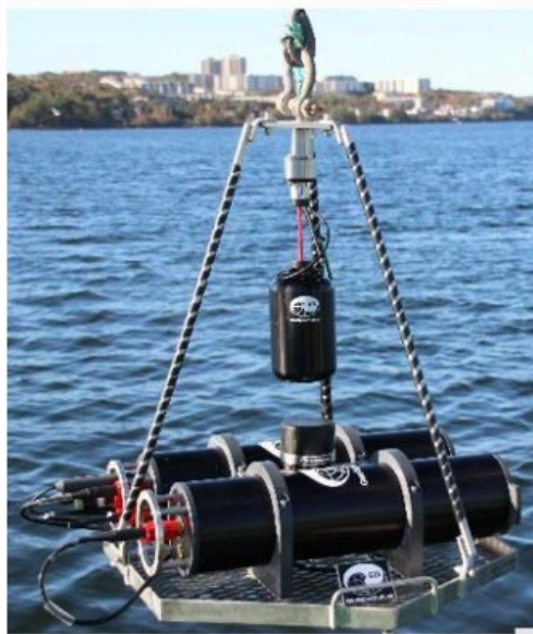
Figure 9. M612-100 particle motion sensor bottom mounted system used as low frequency receiver
