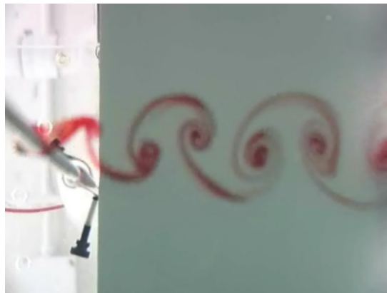
Figure 1.1. Example of low Reynolds number (approx. 200) wake visualization from an overhead view. Source: [4].
