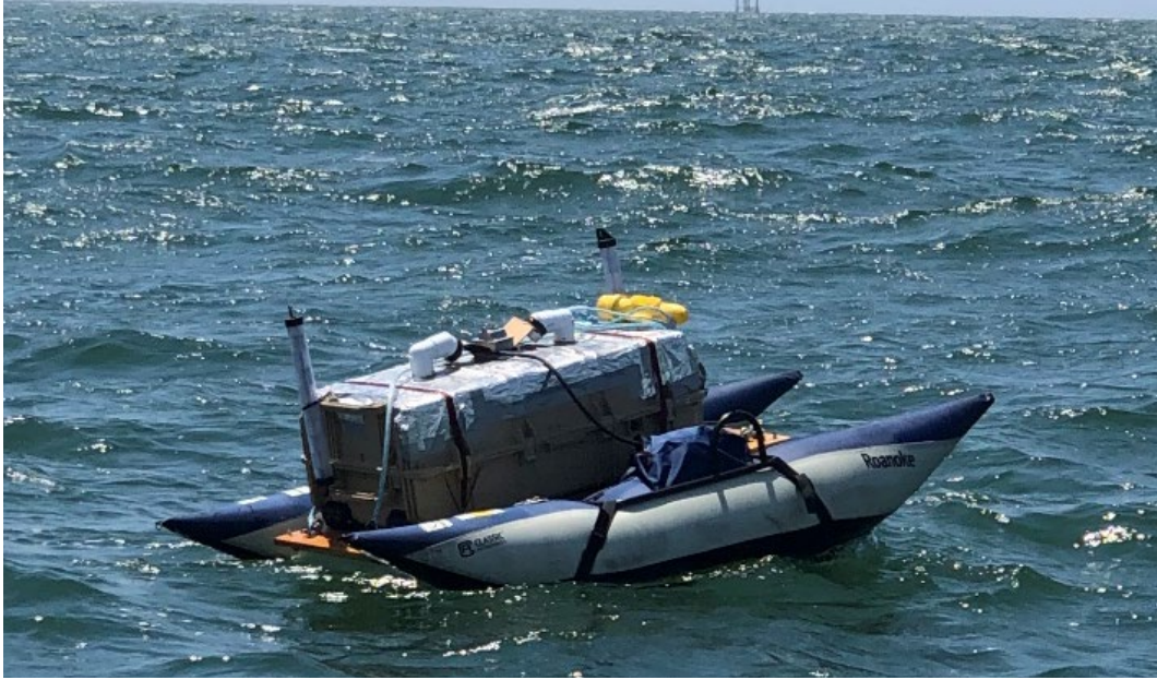
Figure 11. COFFIN on Roanoke pontoon boat after deployment, moored above acoustic source. On each edge of the COFFIN are radar reflectors and an AIS marker to assist in locating the system at the end of each day.
