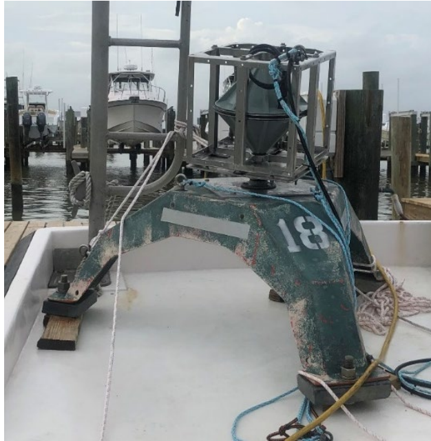
Figure 9. Lubell source on fiberglass mooring. The mooring was held in place with 50 lb weights bolted onto each leg.
