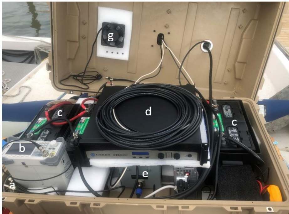
Figure 10. COFFIN interior with a) GPS, b) waveform generator, c) three batteries, d) amplifier, e) Lubell bridge, f) inverter, and g) cooling fan.
