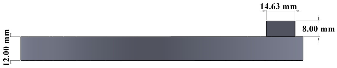
Figure 4. Side View of Cap Design
