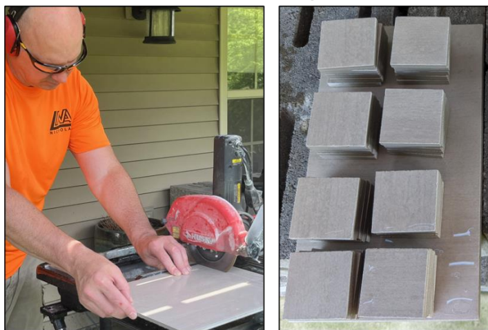
Figure 11. Fabrication of ceramic test coupons used to evaluate the antimicrobial activity of TPX-HL. Remnant restroom tiles being cut with a wet saw (left) and finished 5 \times 5 cm coupons (right).
