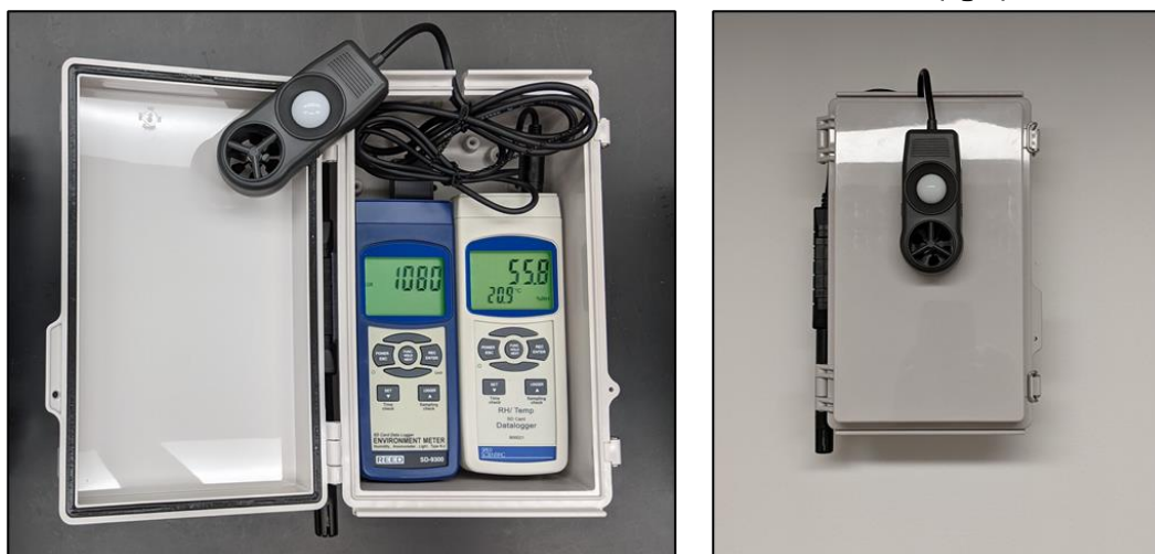
Figure 5. Humidity, temperature, and light data loggers in weatherproof case (left) and loggers mounted on the west wall above the entrance of the restroom (right).
