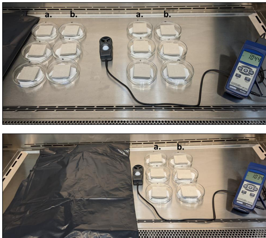
Figure 17. Uncoated and photocatalyst-coated ceramic coupons being irradiated with approximately 1,000 lux florescent light for 17 hr: (a) uncoated, (b) TPX-HL coated, and test specimens incubated in the dark under a black plastic bag (bottom).
