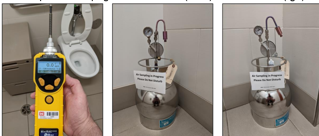
Figure 10. Air sampling for volatile organic compounds (VOCs) using a handheld meter in real time ( left ) and vacuum-pressurized summa canisters. Air samples of 6 L were collected over a 24 hr period. Air sampling in the north restroom ( center ) and south restroom ( right ).
