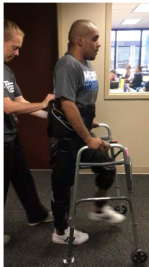
Fig. 2. SCI subject walking with exoskeleton with supplement FES, with assistance from physical therapist.
