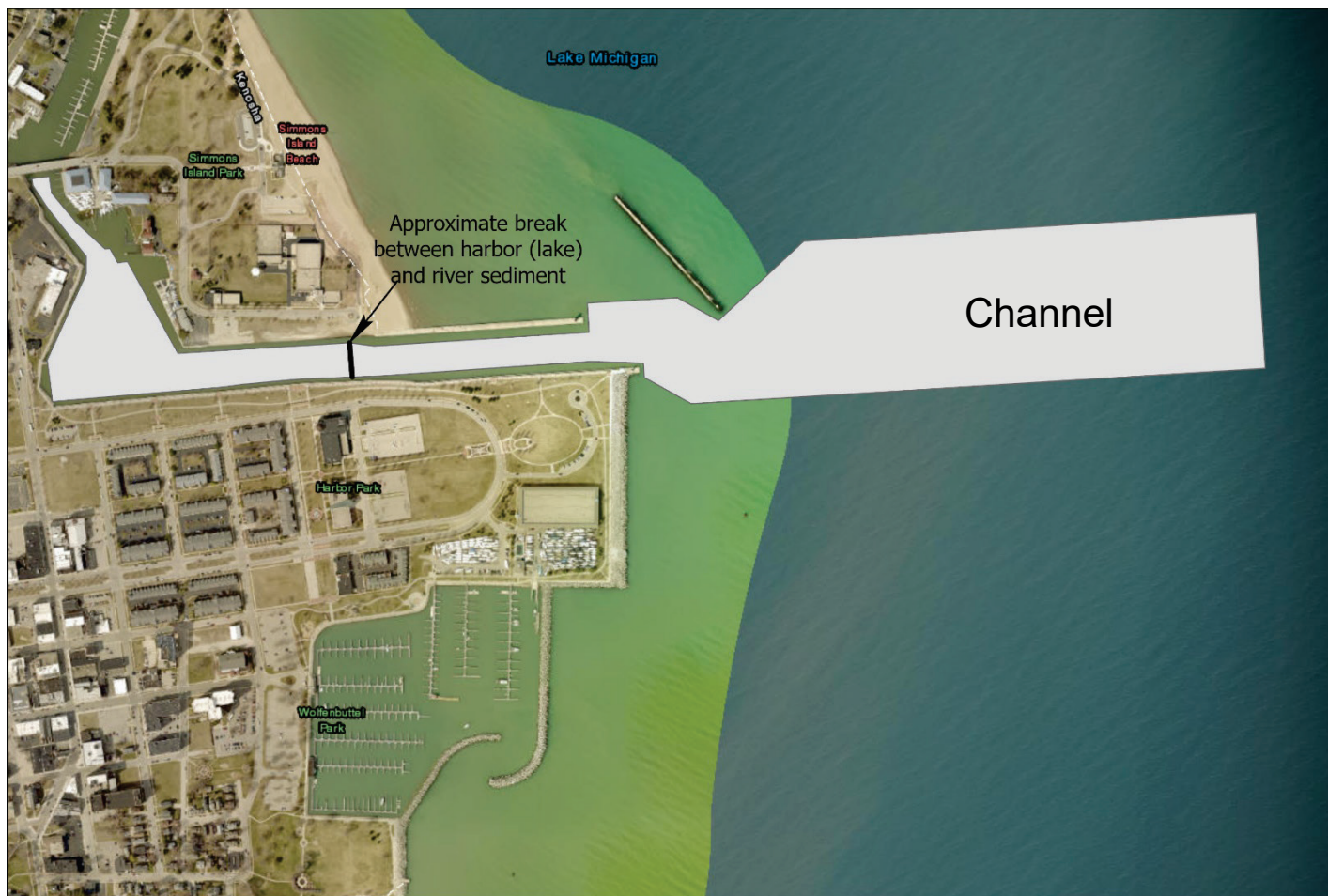
Figure 2. Kenosha Harbor, Kenosha, Wisconsin. Area highlighted in light gray marks the federal navigation channel portion of the harbor and related entrance channel.
