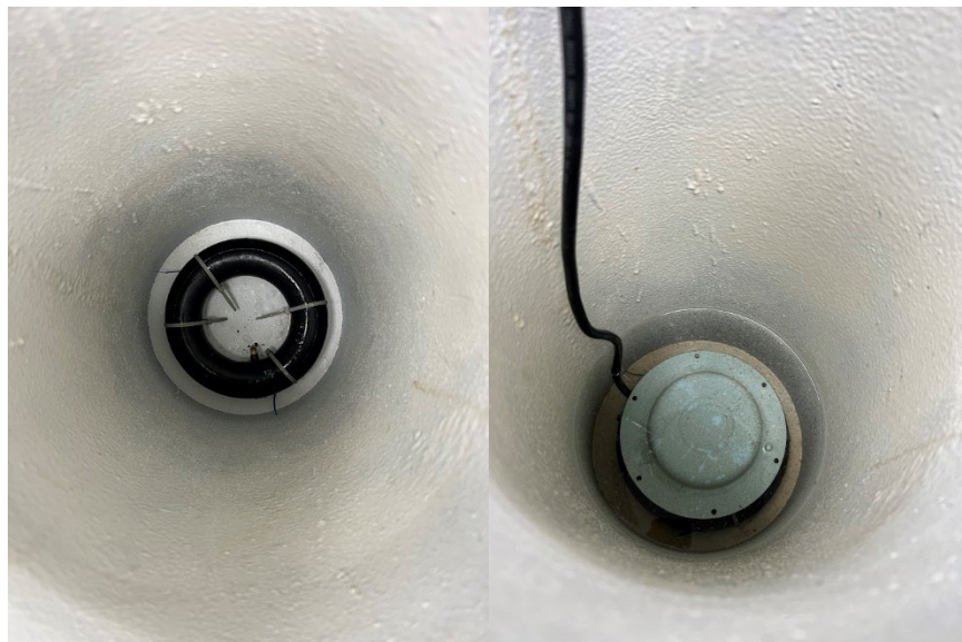
Figure 6. SWT Acoustic Source a) Innertube Dampener and b) Loudspeaker
