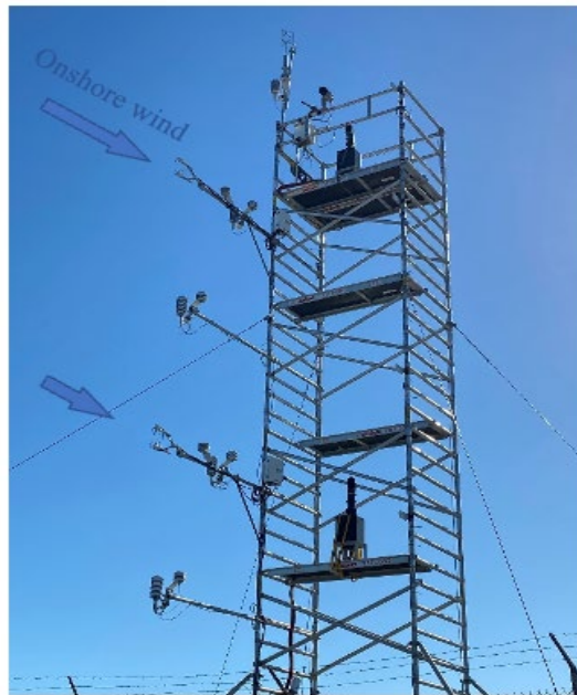
Figure 4. Tower EM0 with all sensors. Onshore wind is illustrated in this figure to denote the orientation of the tower sensors.
