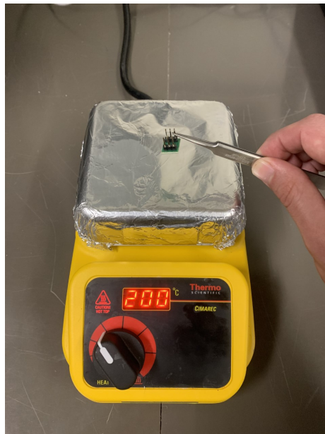
Figure 3.4. Hot Plate used to thermally anneal damaged transistors.
