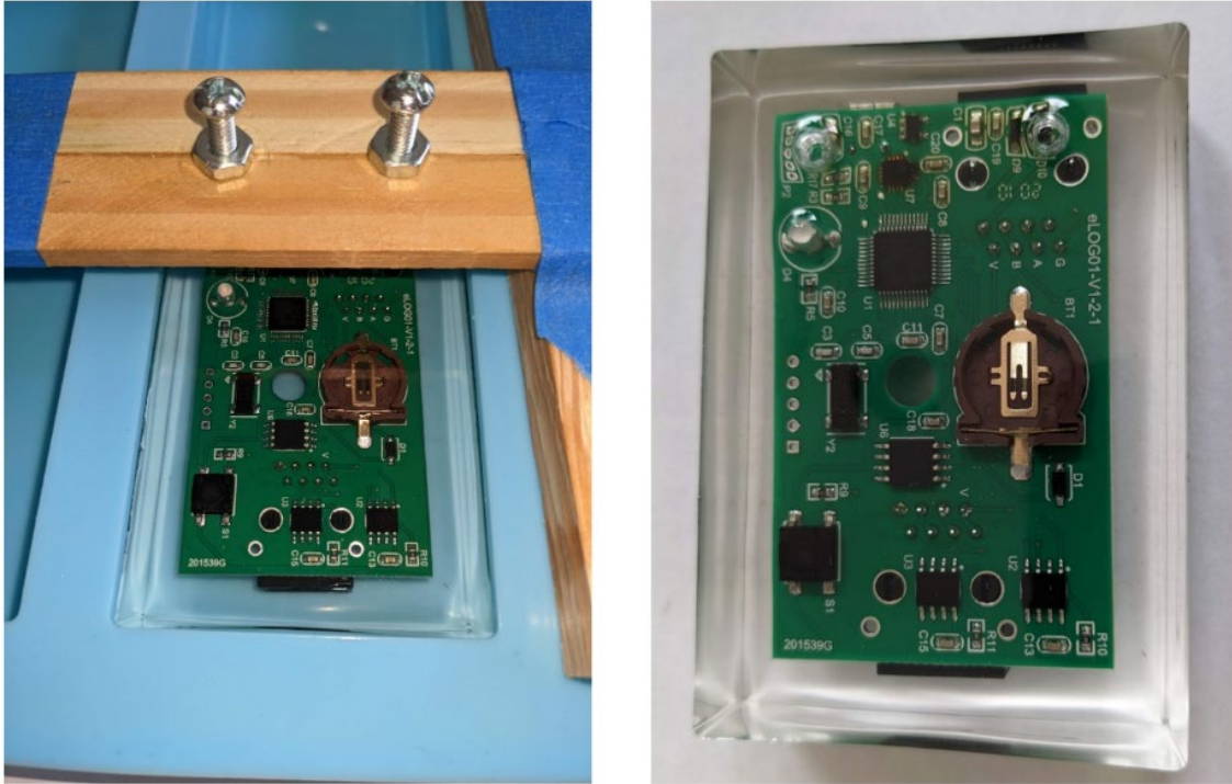
Figure 45. Epoxy-Potted Test PCB Before (L) and After (R) Mold Removal
