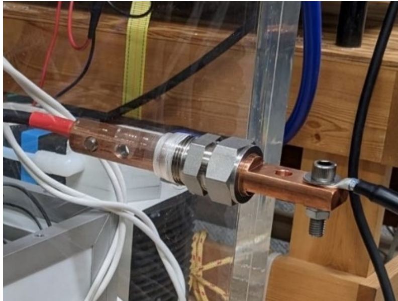
Figure 17. Air Side of Power Feedthrough Assembly Installed in Vacuum Chamber Wall
