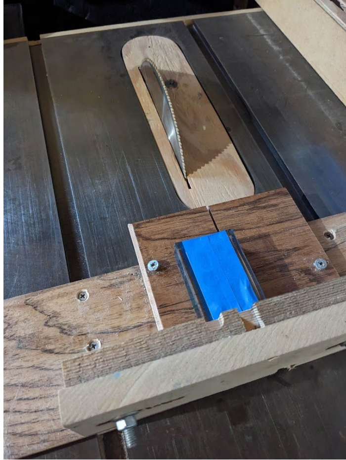
Figure 46. Removing Excess Potting Material with Table Saw
