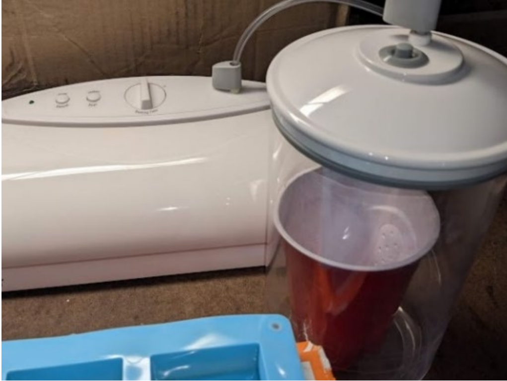
Figure 44. Epoxy in Vacuum Chamber to Remove Air Bubbles
