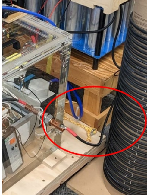
Figure 29. Positive Cable from Air-Core Inductor to Power Feedthrough for Switching Test
