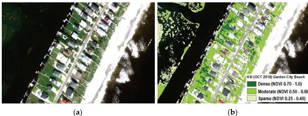
Figure 3. National Coastal Mapping Program (NCMP) Hyperspectral Image (a) and the NCMP-derived vegetation density data (b), where categories include Dense vegetation (NDVI values 0.70–1.0), Moderate vegetation (NDVI values 0.50–0.69), and Sparse vegetation (NDVI values 0.25–0.49).
