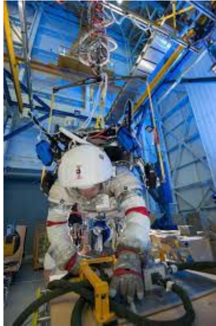
Figure 2.10. An engineer testing an astronaut suit using ARGOS. Source: [17].
