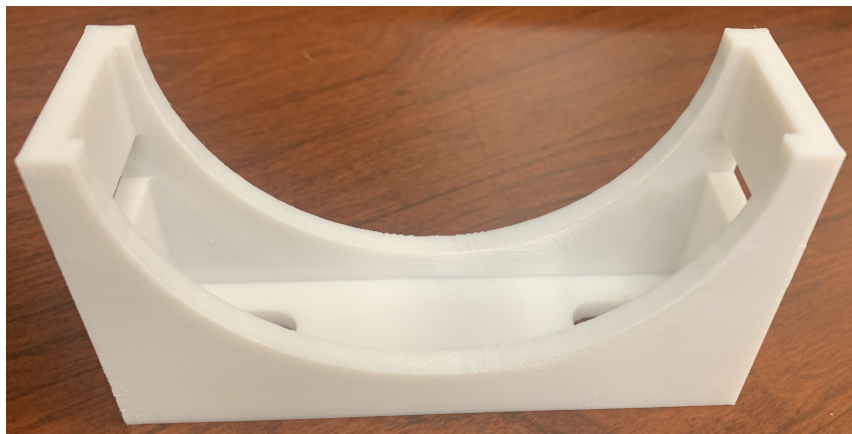
Figure 8.6. One of the two AM air tank supports.
