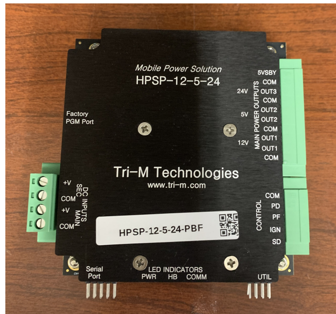
Figure 6.11. HPS3524 power supply unit.
