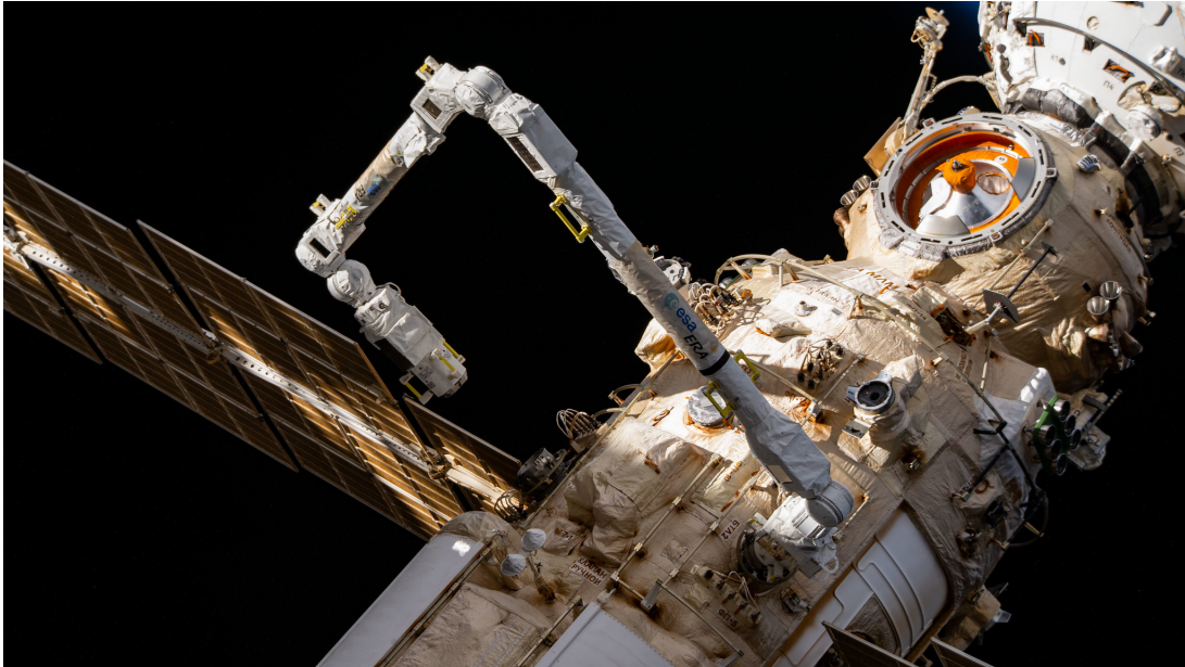
Figure 2.12. The ERA operating on the Russian side of the ISS. Source: [22].
