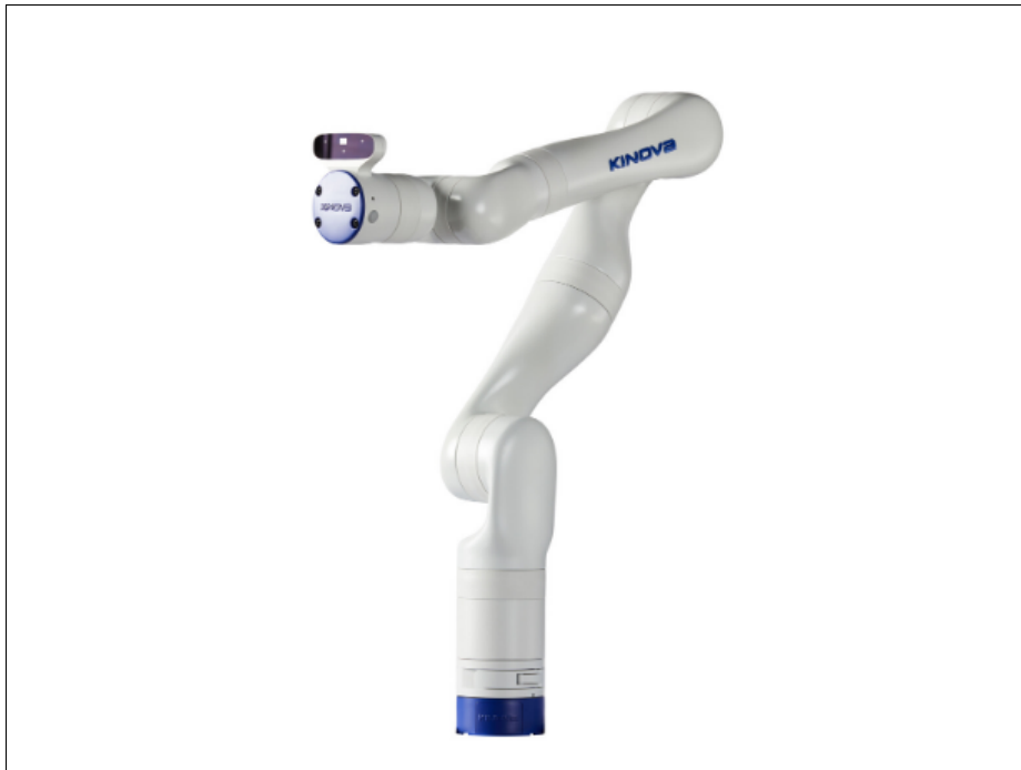
Figure 6.15. Kinova Gen3 Ultra lightweight robot. Source: [45].
