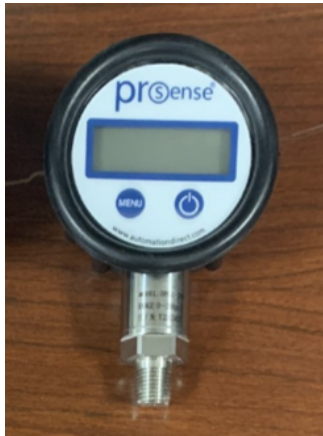
Figure 7.7. ProSense DPG1-5000 digital pressure gauge.
