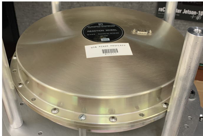
Figure 6.5. 20.3 N-m-s reaction wheel mounted on the middle plate.
