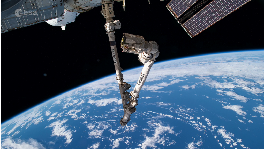
Figure 2.11. Canadaarm 2 attached outside the ISS. Source: [20].
