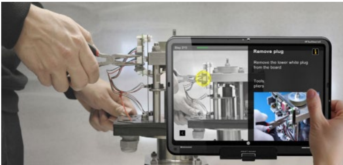
Figure 9. An Example of “Adaptive Visual Aid.” Source: Webel et al. (2013).
