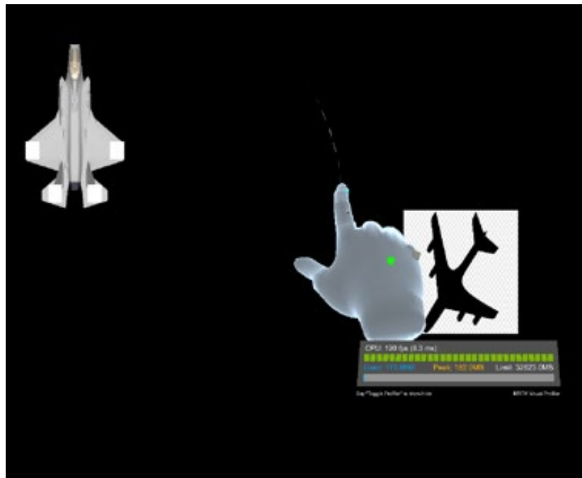
Data Source: image received from Ezra Idy from NAWCAD RISE Lab on March 15, 2023. The interface display in the top left of the image was ultimately discarded because the display would impede the user’s vision when conducting towing operations.
