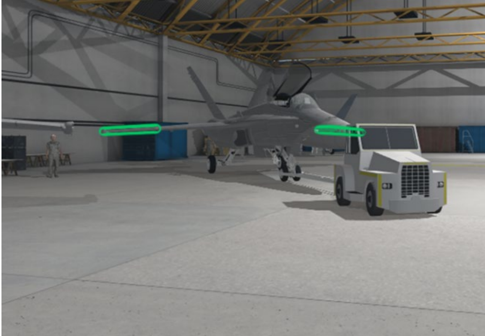
Figure 13. AR Collision Interface Wing Tip Indicators. Source: Fetterolf (2020).
