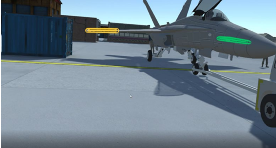
Figure 14. AR Collision Interface Interacting with Occluded Wingtip. Source: Fetterolf (2020).
