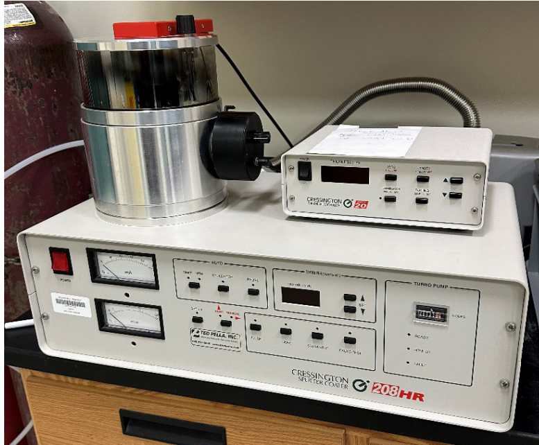
Figure 9. Cressington Sputter Coater 208HR
