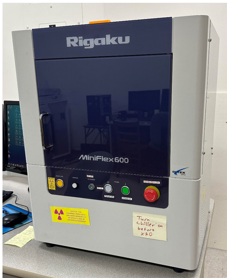
Figure 14. Rigaku MiniFlex 600 X-Ray Diffractometer
