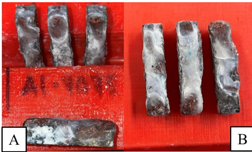
Figure 25. Images of Al-7075 Showing Salt Covered Samples after a) 6 Weeks and b) 12 Weeks.
