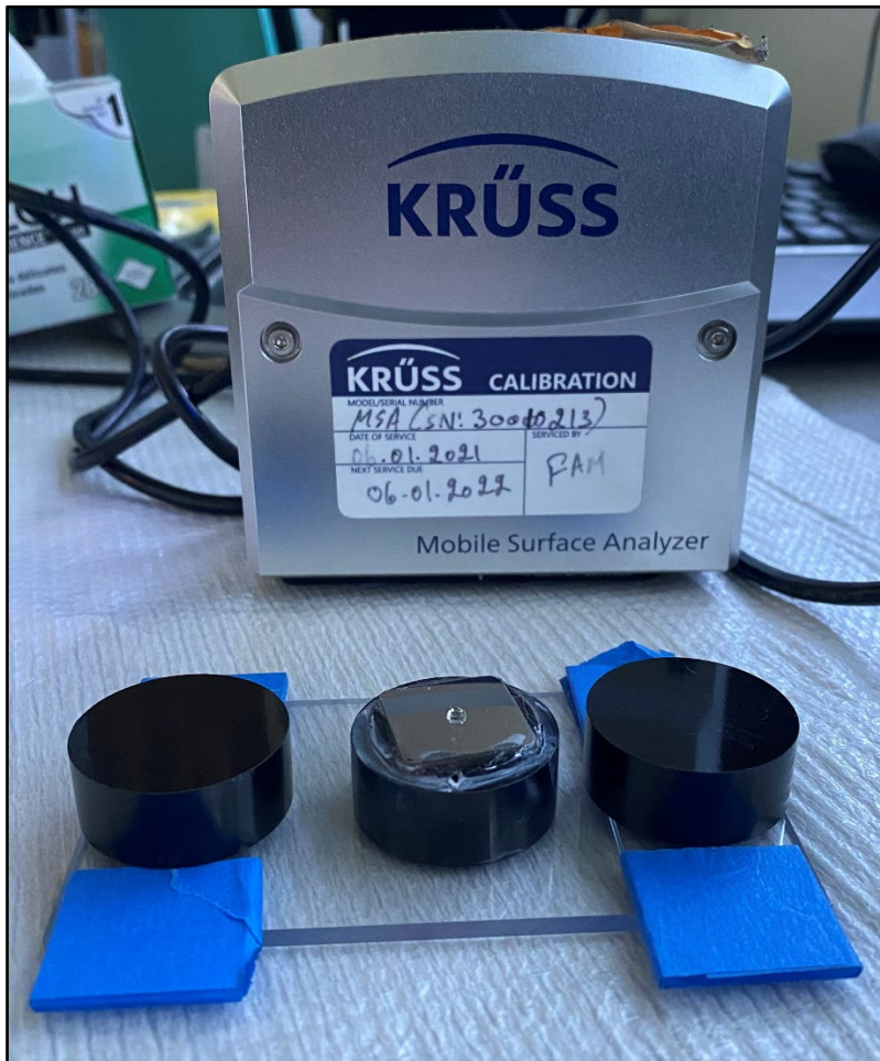
Figure 48. Krüss MSA Measurement Setup Modifications for Polished Surfaces.
