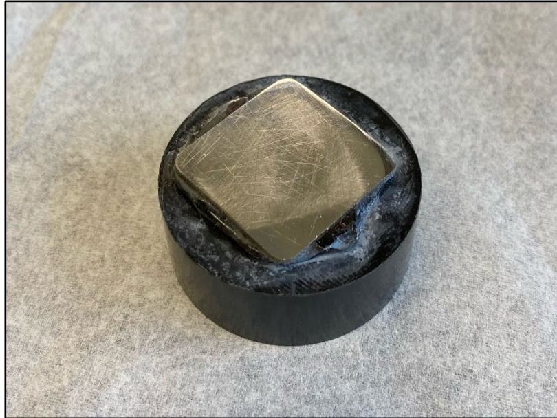
Figure 47. Externally Mounted Print Sample for Grinding/Polishing Process.
