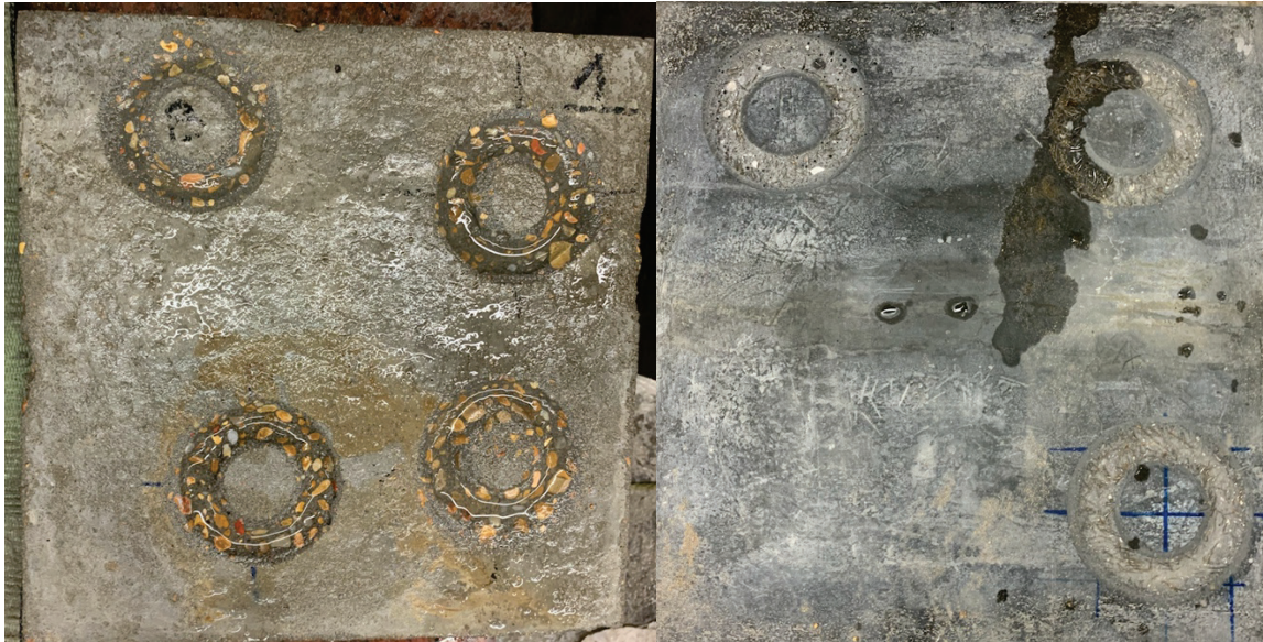
Figure 28. ASTM C779 (2019c) abraded surfaces of PAC-5 ( left ) and Lock-Tuf ( right ).
