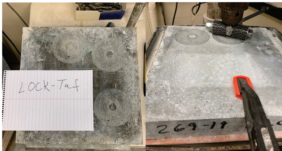
Figure 32. Typical abrasion of Lock-Tuf in ASTM C944 (2019b) rotating-cutter method.
