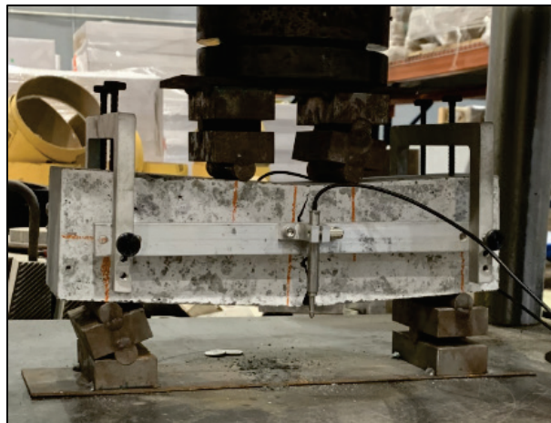
Figure 13. ASTM C1609 (2019d) flexural performance test.
