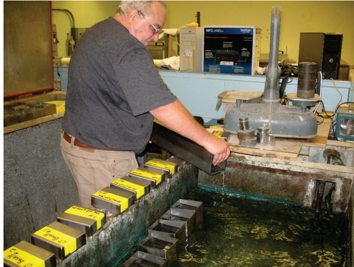
Figure 14. ASTM C666 (2015) freeze–thaw testing.
