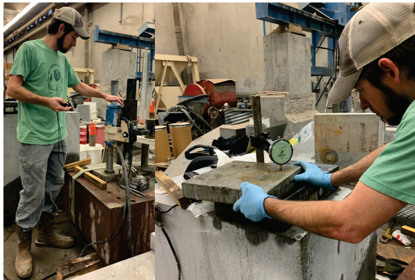
Figure 19. ASTM C779 (2019c) core barrel abrasion testing.
