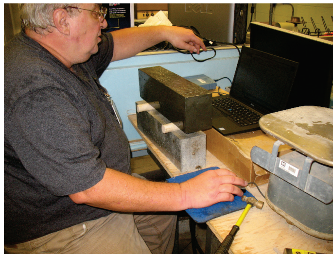
Figure 15. Relative dynamic modulus testing of a freeze–thaw beam.
