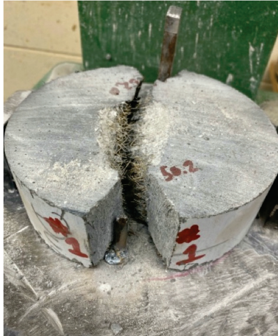
Figure 34. Impact test of a Lock-Tuf sample.
