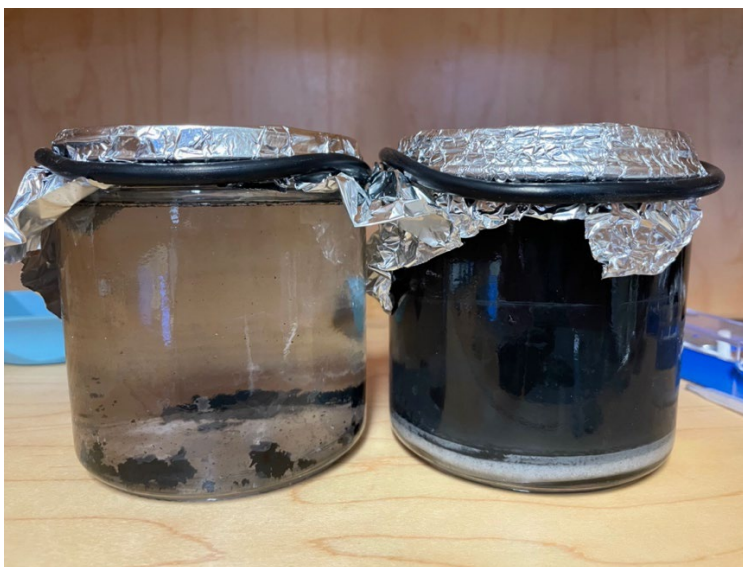
Figure 14. Left DI water CNT suspension, right PVA 1.5 wt.% CNT suspension
