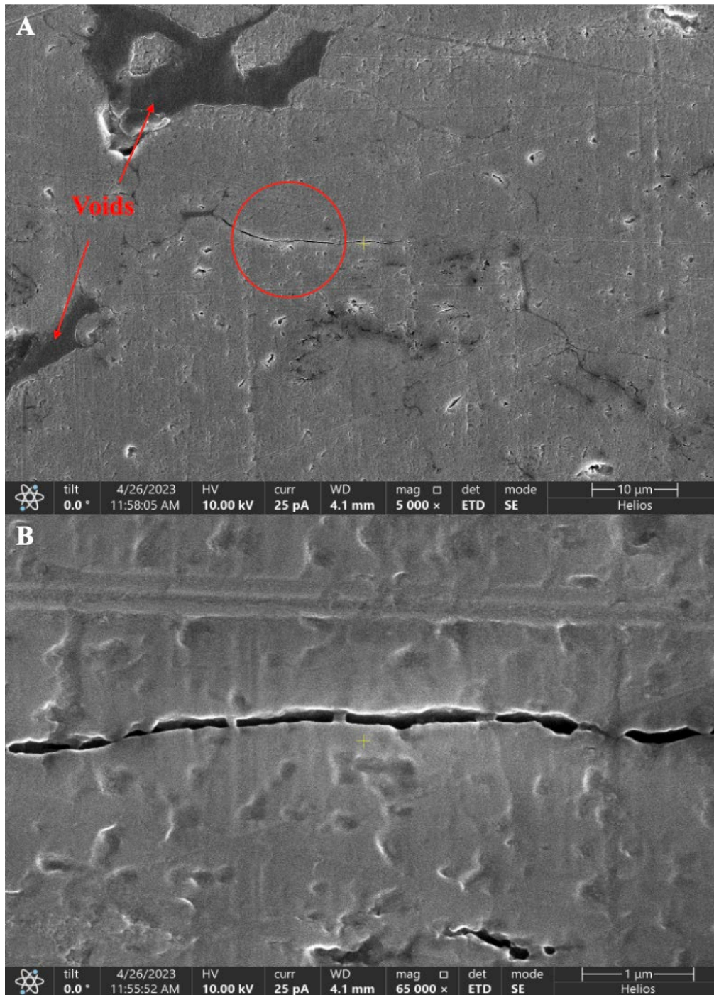
Figure 29. Pure Al coating series of splat boundaries with no reinforcements a) splat boundary circled b) high magnification splat boundary
