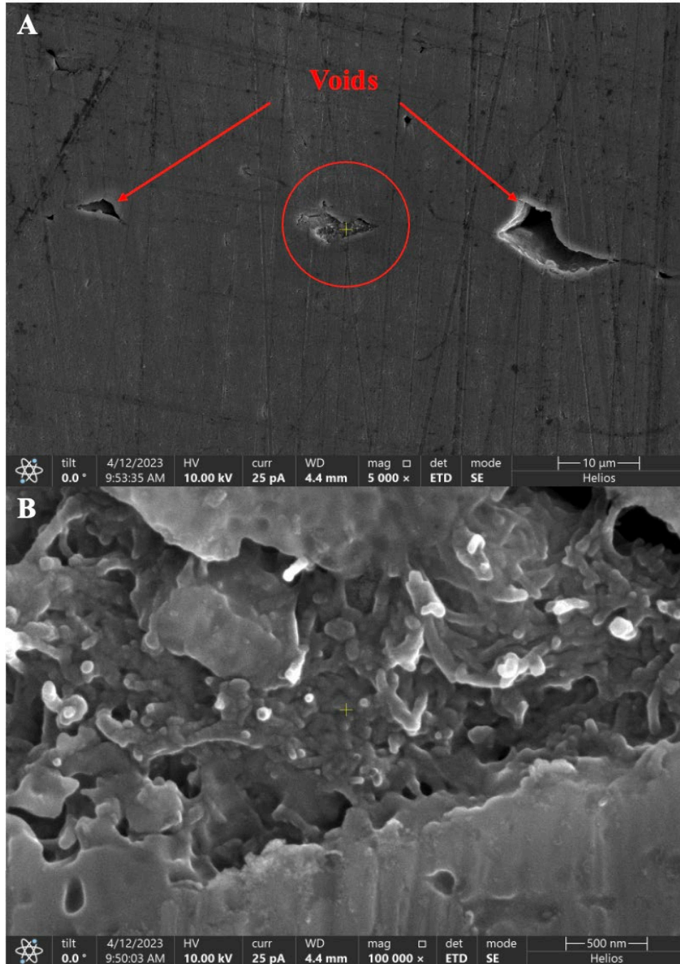
Figure 30. HEBM CS coating 3 vol% CNT a) CNTs in splat boundary circled b) high magnification of CNTs in splat boundary
