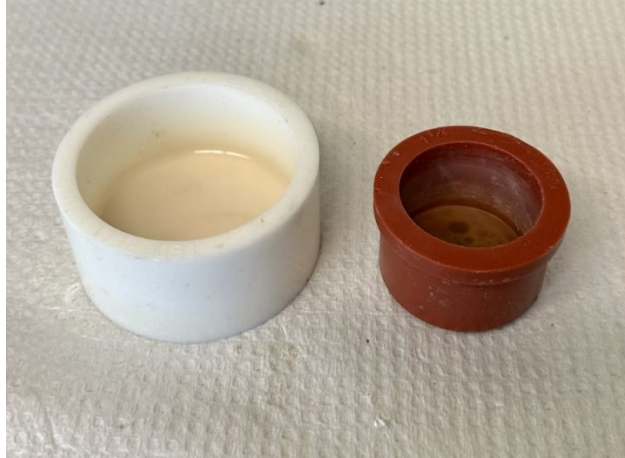
Figure 5. The two molds that were used in the molding fabrication process
