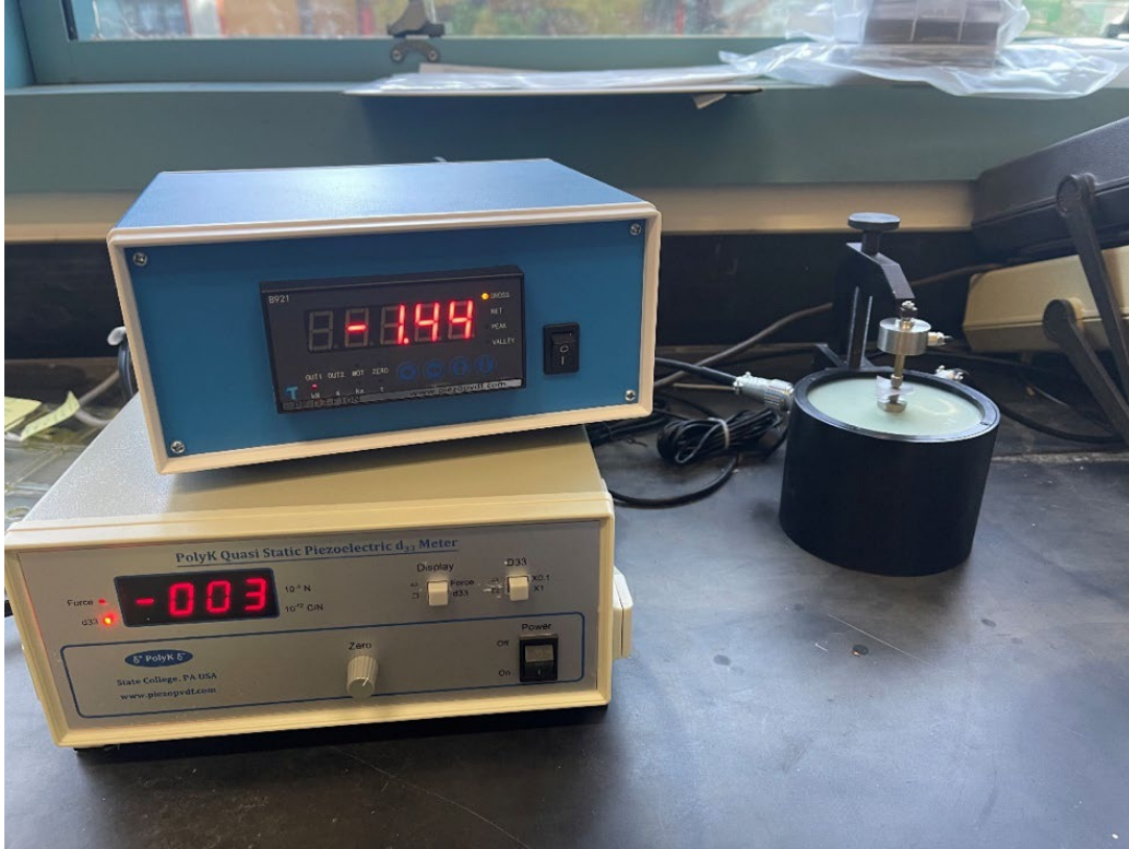
Figure 9. Testing devices (shown counterclockwise from bottom): PolyK Berlincourt piezoelectric d_{33} meter, static force meter, and sample holder
