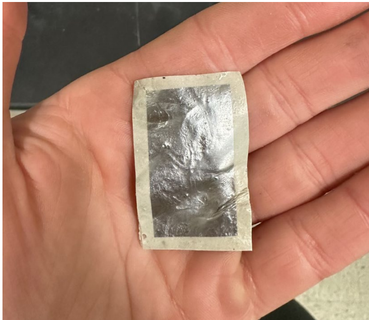
Figure 11. The sample after the sputter coating process was conducted with Scotch tape.
