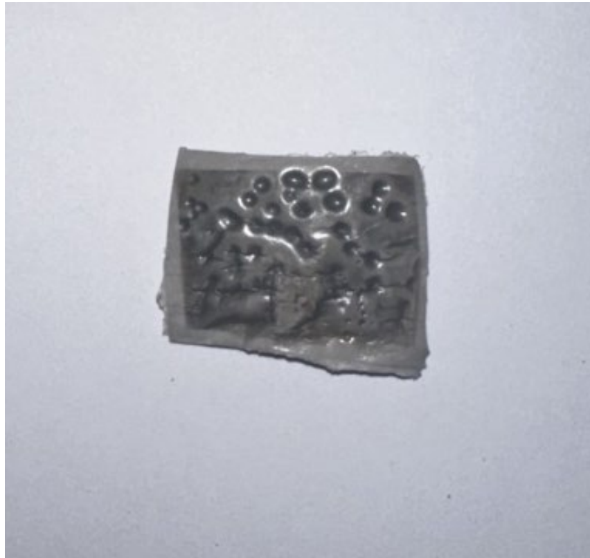
Figure 12. The surface imperfections of the second molded film
