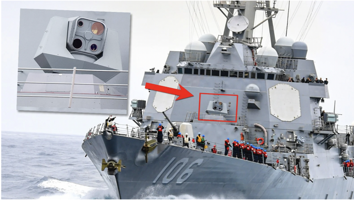
Figure 2.3. ODIN System Installed on USS Stockdale (DDG 106). Source:[2].
