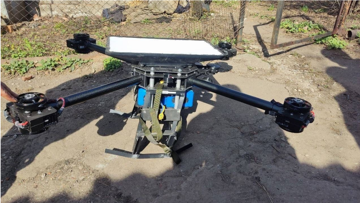
Figure 2. Ukrainian UAV Used to Drop 82mm Mortar Rounds Equipped with a Starlink Terminal Captured by Russian Forces. 60
