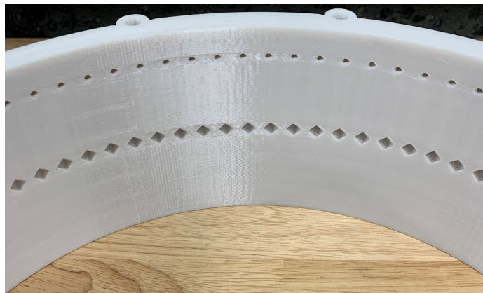
Figure 3.15. Polycarbonate Passage Inlet and Exit Manufacturing Quality
