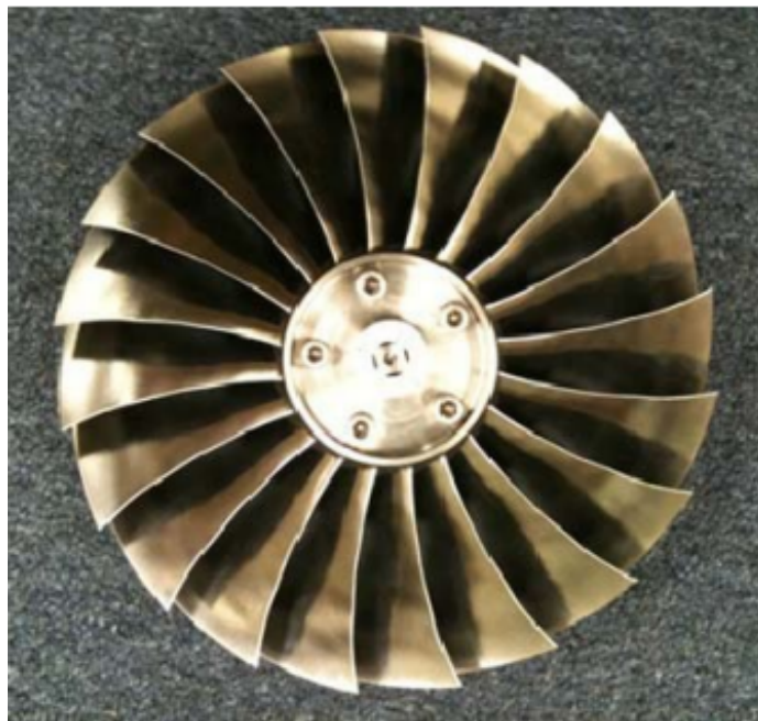
Figure 2.2. The NPS Military Fan Blisk. Source: [7]
