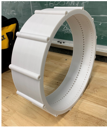
Figure 3.13. IP Polycarbonate Casing
