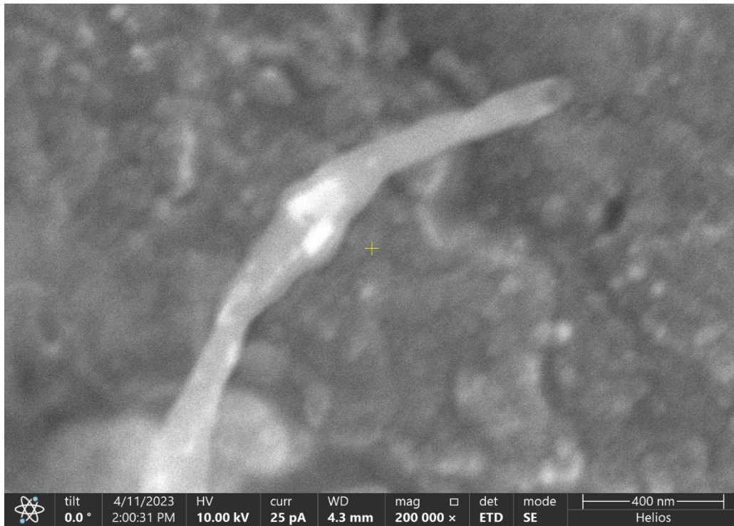
Figure 42. SEM image of individual BNNT located in coating 1
