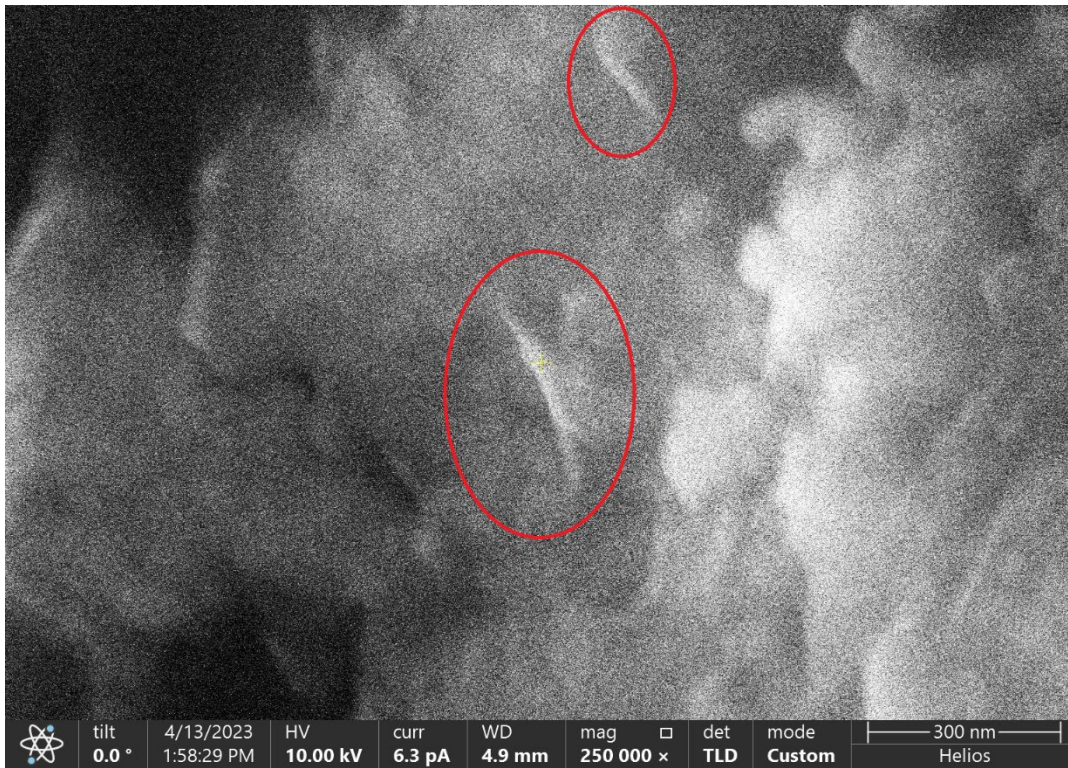
Figure 50. Top-down SEM image of BNNTs located in coating 2
