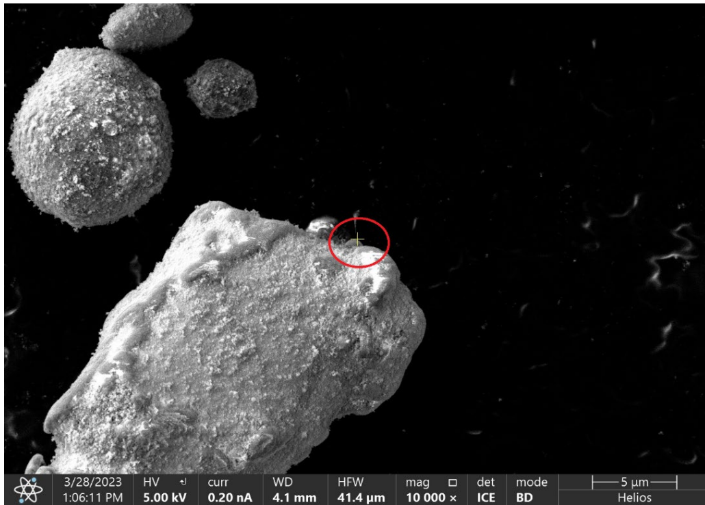
Figure 30. BNNT location on Al-7075 particle
