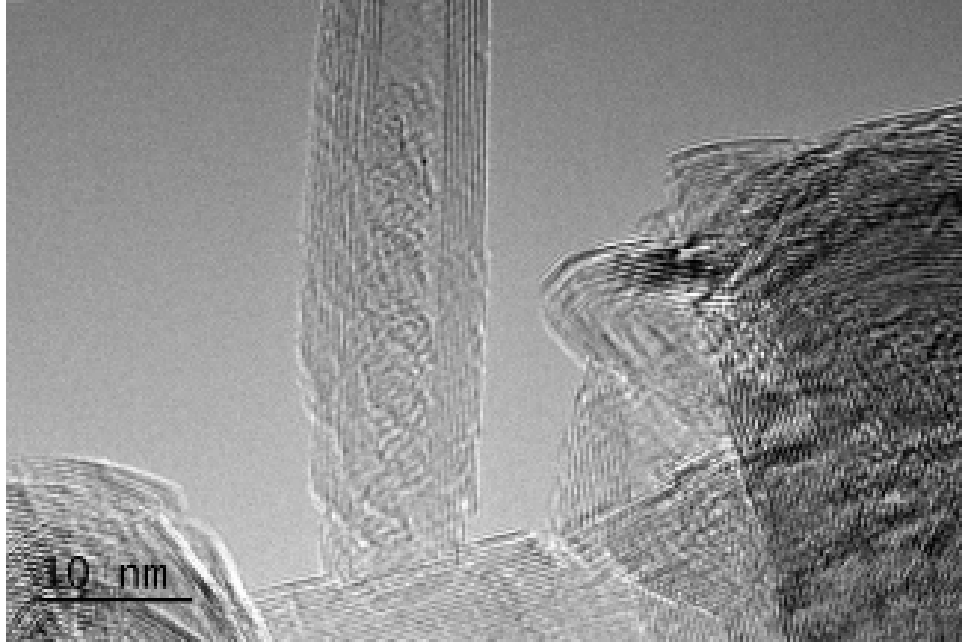
Figure 12. TEM image of a BNNT, as received from the manufacturer. Source: [3].
