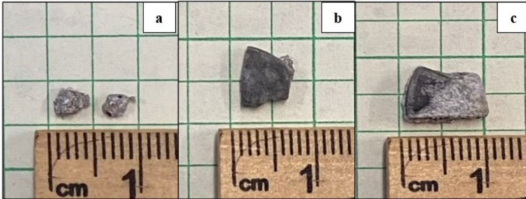
Figure 21. 1600°C for 1 hour pre-mounting images: (a) HEB (B1), (b) HfB 2 (H1), and (c) ZrB 2 (Z1).
