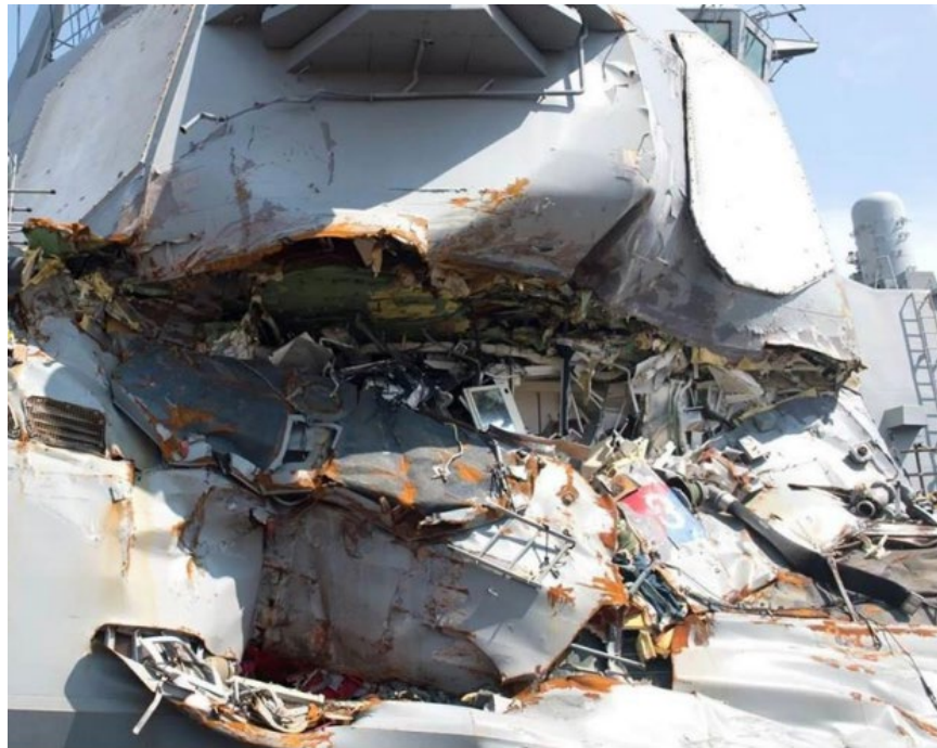
Figure 4. USS Fitzgerald Collision Damage. Source: Department of the Navy (2017).
