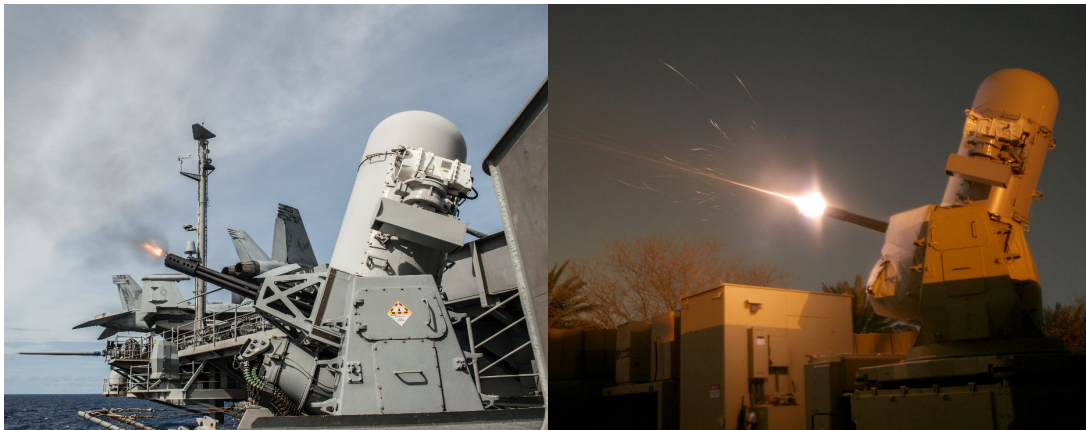
Figure 35. Autonomous Afloat and Onshore Weapon Systems. Phalanx CIWS Weapon System (left). Source: N. Burke (2016). Phalanx C-RAM Weapon System (right). Source: United States Army Acquisition Support Center (USAASC) (n.d.).
