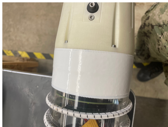
Figure A.5. Aft Section of DREW UV Shown Wrapped with Polyken Tape at Aft Seam
