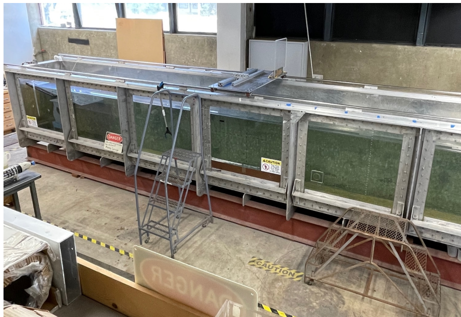
(b) Tow Tank Side View
