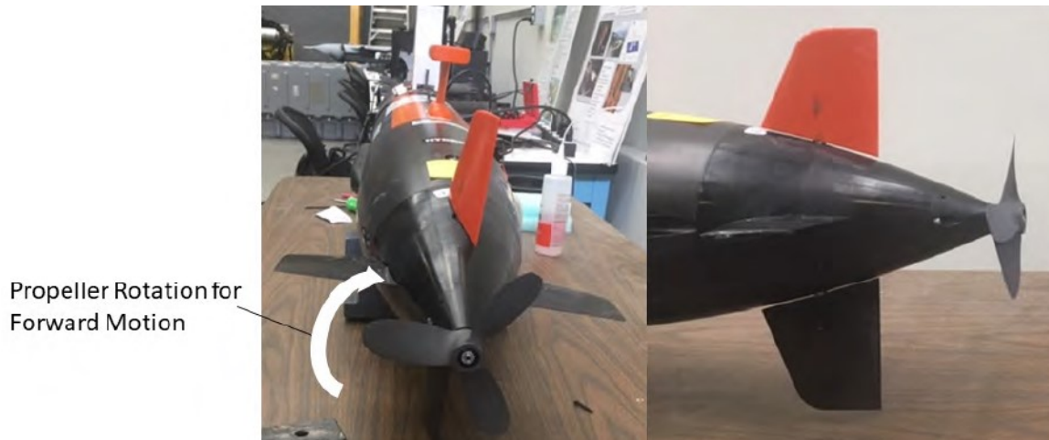
Figure 1.4. REMUS 100 Three-Bladed Propeller without Shroud. Source: [3].
