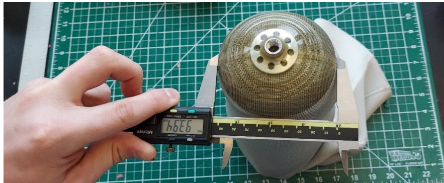
Fig. 17. Measurement of umbrella diameter for use in ferrous liner fabrication.
