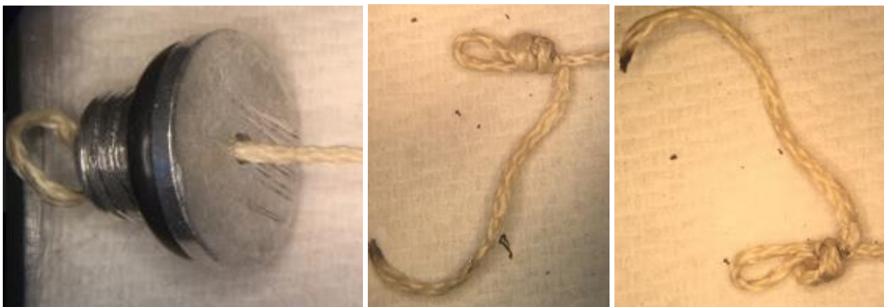
Fig. 23. Figure 8 on a bight knot after testing 25,000 cycles at 120-140 N max force.
