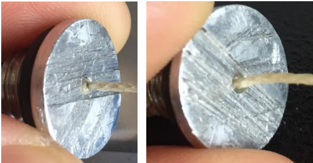
Fig. 20. Knot slippage. Left image: Knot slipping through the hole that holds the tether. Right image: Knot sitting above hole and not pulling out.
