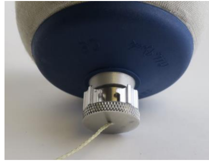
Fig. 33. Quick Pin final design. The user rotated the yellow knob, slid the pin into the slot, and then released the yellow knob to lock the pin in place.
