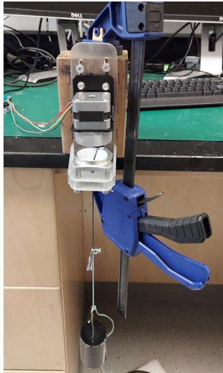
Fig. 24. Tether testing setup. The tether was run through the tether guide, and weights were hung at the bottom. There was a motor at the top of the apparatus that applied rotations to the tether.
