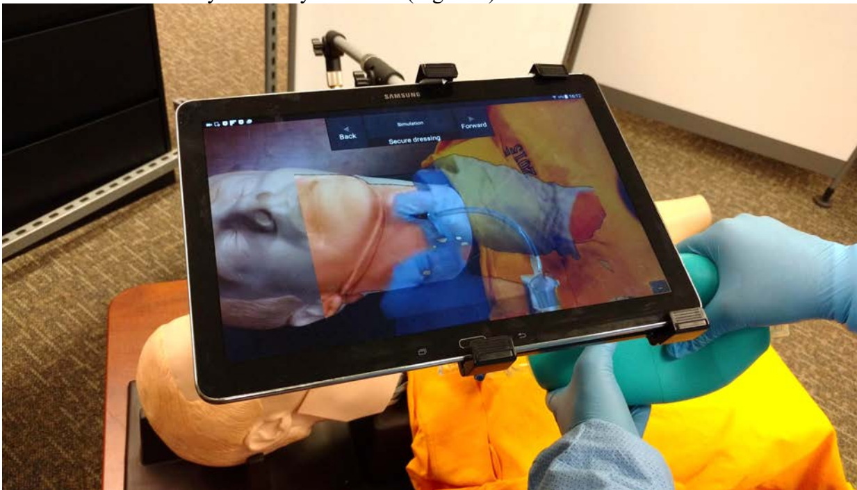
Figure 3. The display overlays a visualization of a future step of a cricothyrotomy procedure onto the simulator.
