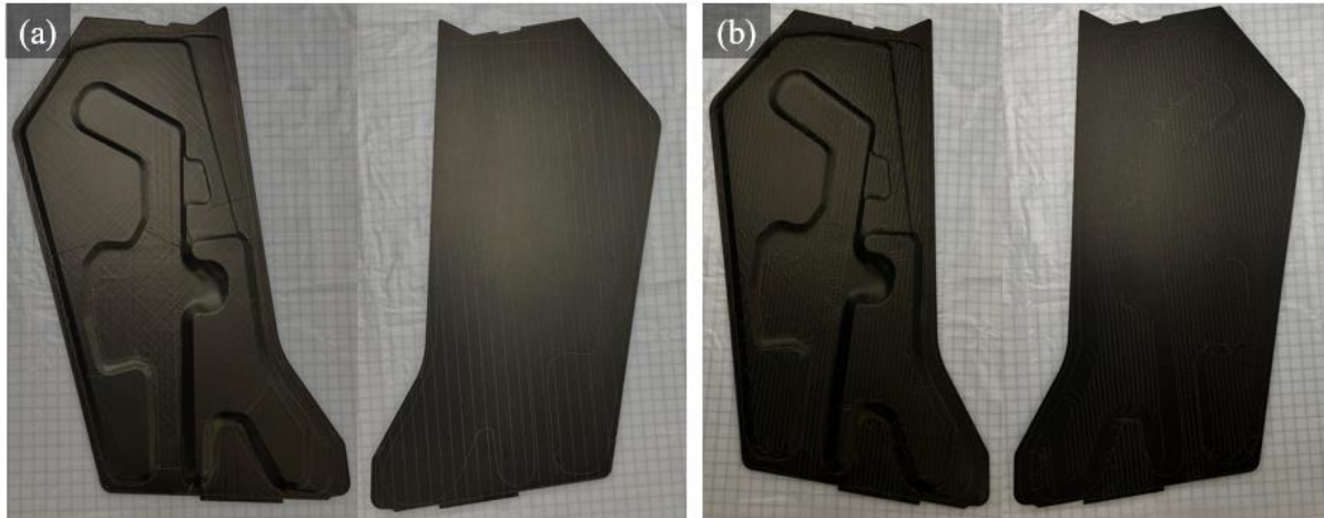
Figure 60. Post-cure and trim of (a) SD1 with perimeter stitching and (b) SD2 with perimeter and through foam stitching
