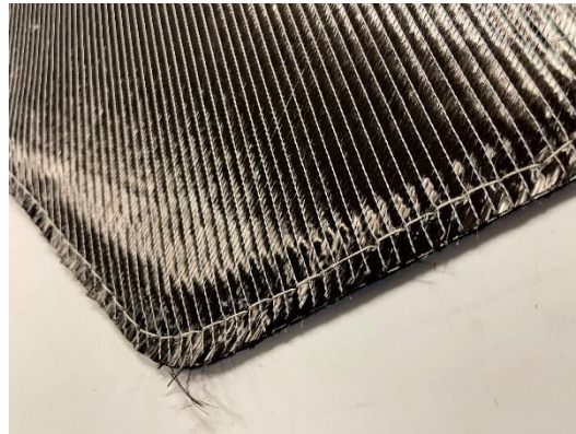
Figure 53. Exterior Stack Perimeter Stitching
