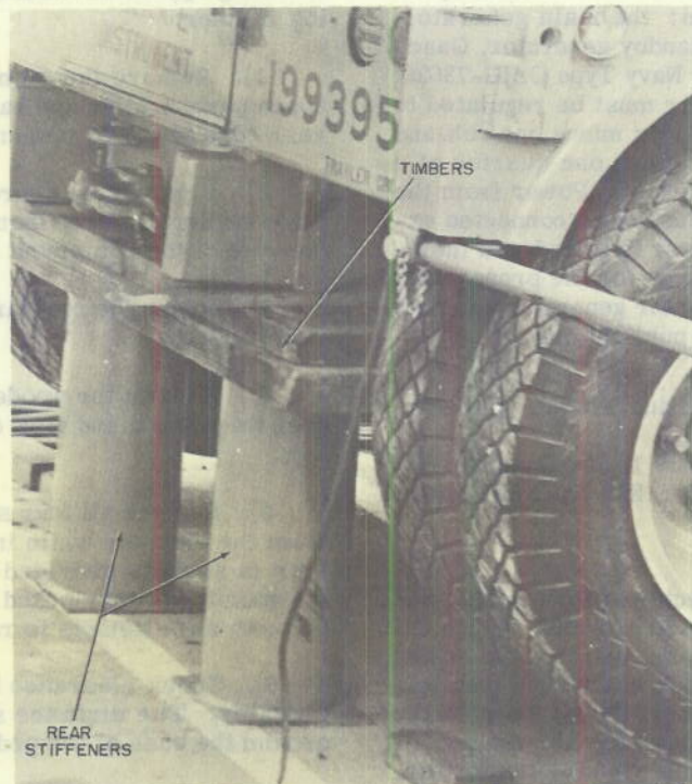
Figure 5-5. Rear Stiffeners and Timbers Under Rear Crossmember of Equipment Trailer
