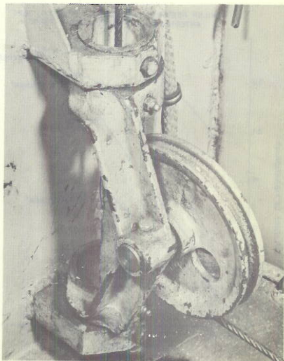
Figure 3-99. Sheave in Antenna Elevator With Larger Shaft
