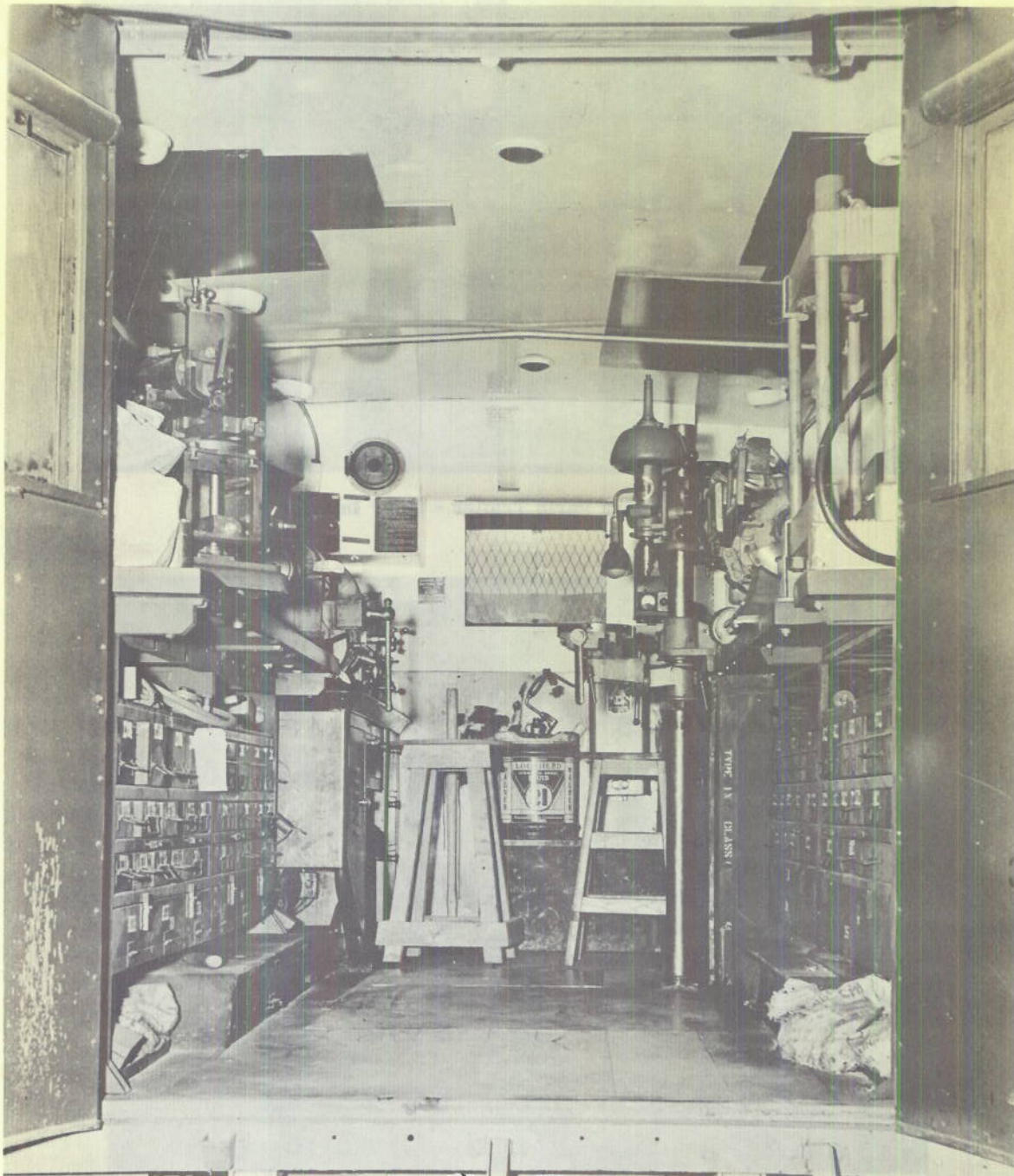
Figure 3-112. Machine Shop Truck - Interior View
