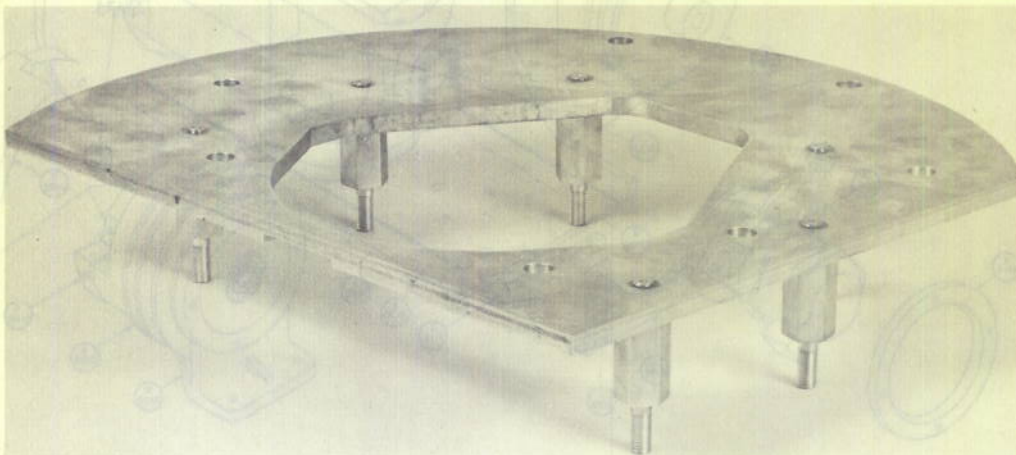
Figure 3-88. Dural Mounting Plate for Nutator Motor (Back of Antenna)
