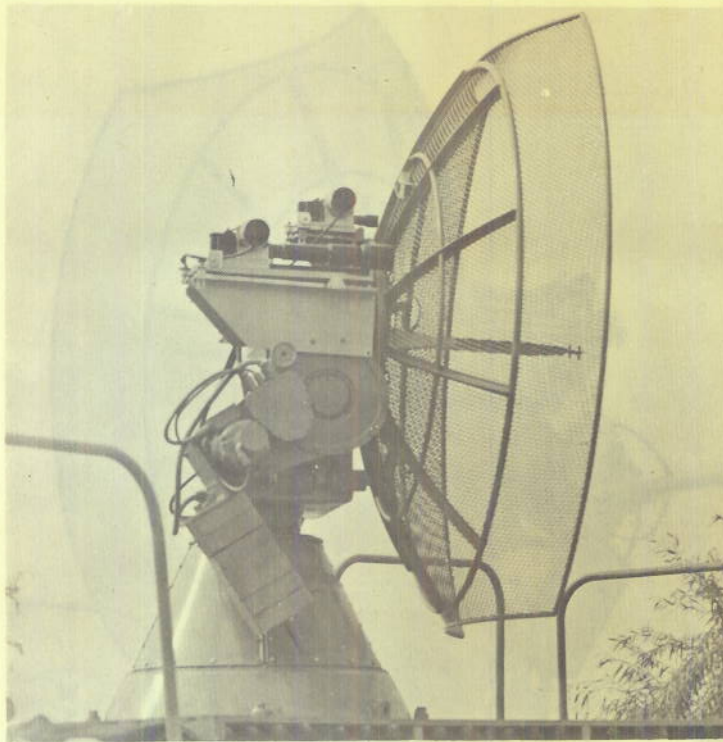
Figure 3-80. Antenna Unit - Left Side View Showing Cameras, Elevation Motors, Counterbalance, and Pedestal
