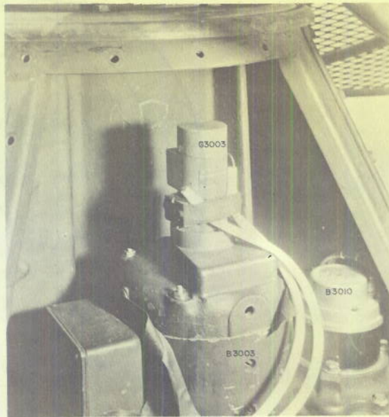
Figure 3-82. Antenna Train Motor and Tachometer in Pedestal
