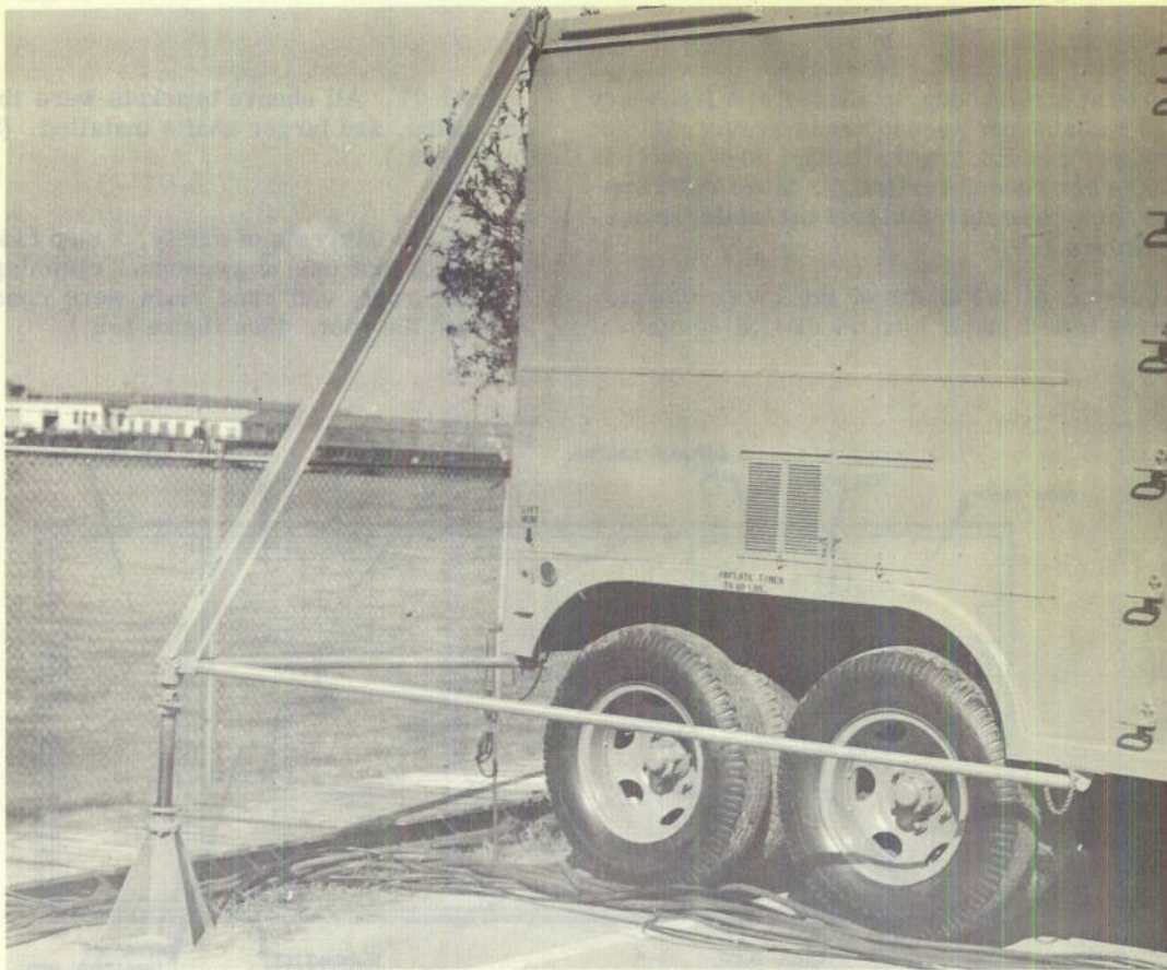
Figure 3-97. Outrigger and Jack for Equipment Trailer
