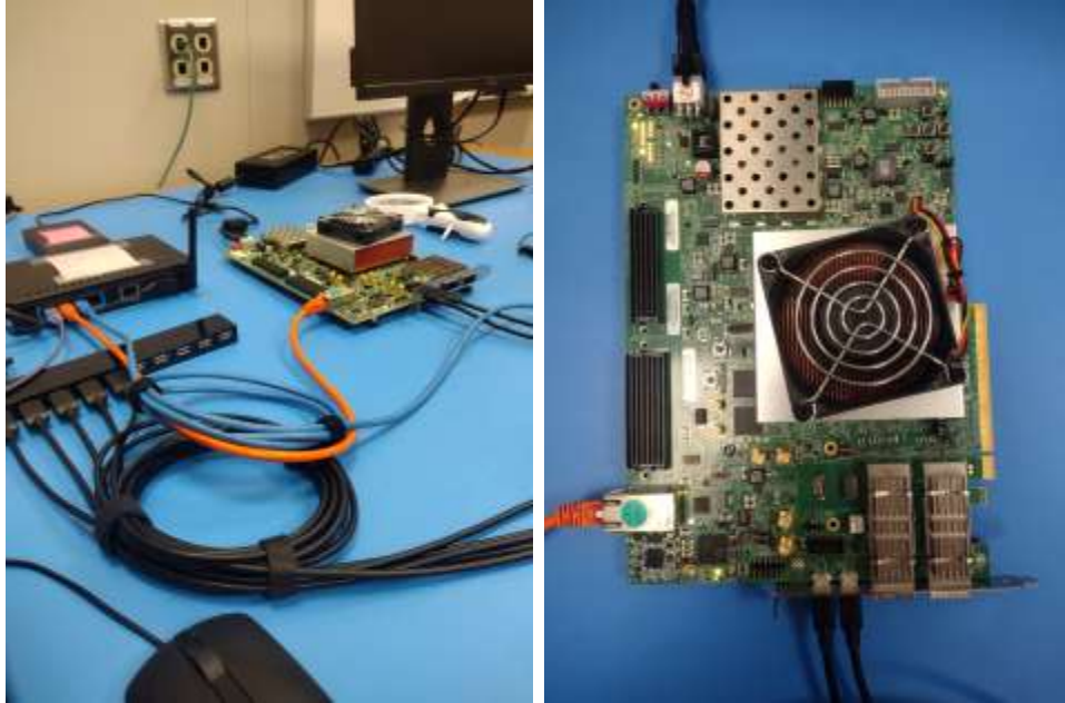
FPGA Dev Board Xilinx VCU118 connected to host. Booting Linux on RISC-V core and then running application, invoking the accelerator.
