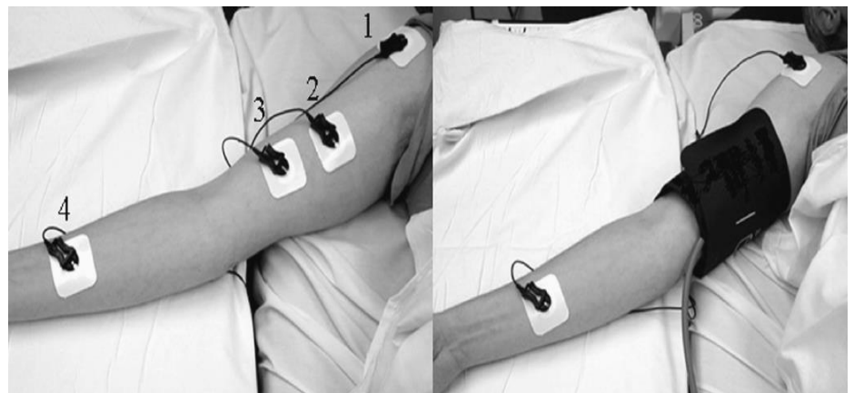
Figure 7: Orientation of electrodes used for tetra-polar impedance plethysmography. Electrodes 1 and 4 inject current toward electrodes 2 and 3, respectively. Ward et al 2010.
