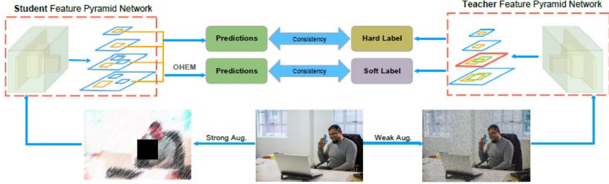
Figure 16: Overview of CrossMatch . CrossMatch enforces consistency between different scales of feature maps. The teacher model takes weakly augmented images and produces artificial (in both soft and hard form, with a refined OHEM employed for the regions used for soft) with a heuristically selected level of features (denoted by red). The student model takes strongly augmented images and constantly makes predictions with every level of the feature pyramid . The consistency constraint is enforced through both soft and hard pseudo-labels.
