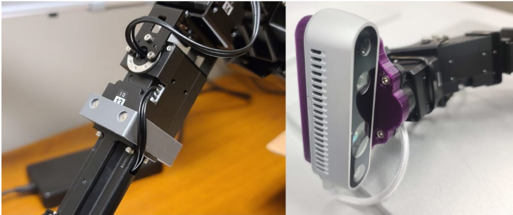
Figure 3. The 3D-printed 90-degree servo mount ( left ) and 3D-printed camera holder ( right ).
