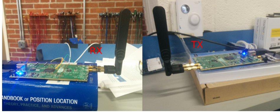
Fig. 13 The USRP B200 devices used for experimentation
