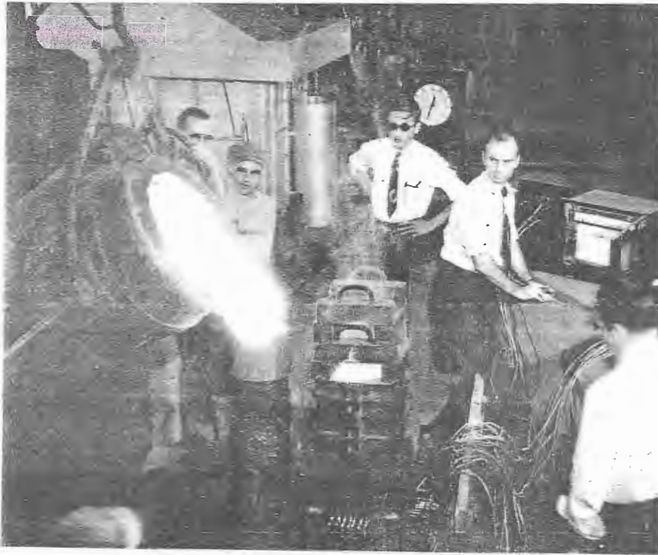
Pouring an experimental ingot in the Naval Research Laboratory Foundry. By the use of thermocouples and automatic potentiometer recorders, complete temperature records are made of the metal and mold throughout the pouring and solidification period.
