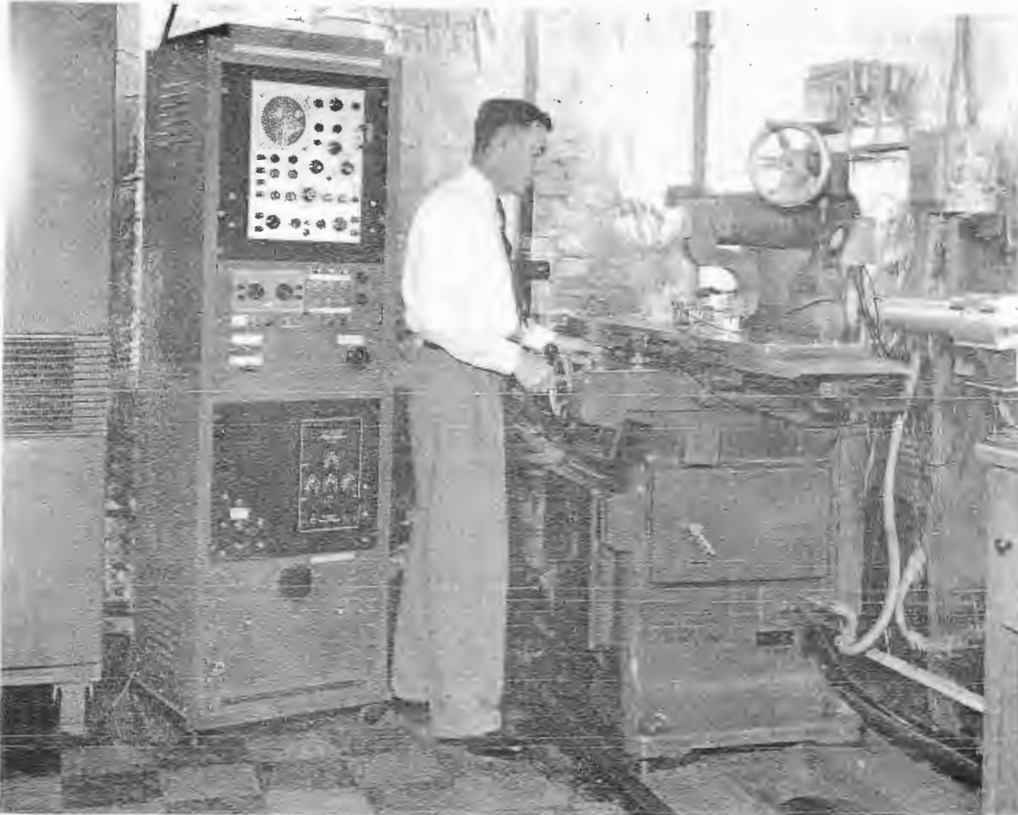
This stick-slip machine has been developed at the Laboratory by rebuilding a standard machine tool. With it the lubricating action of lubricants on various metal surfaces can be examined and, by the use of electronic and optical-photographic methods, records are obtained for later study and comparison with other lubricants or metal surfaces.
