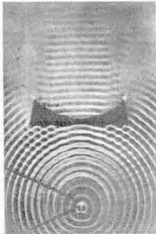
A phase-front pattern made by the ripple tank. The probe-vibrator which excites the water is seen in the lower left.
