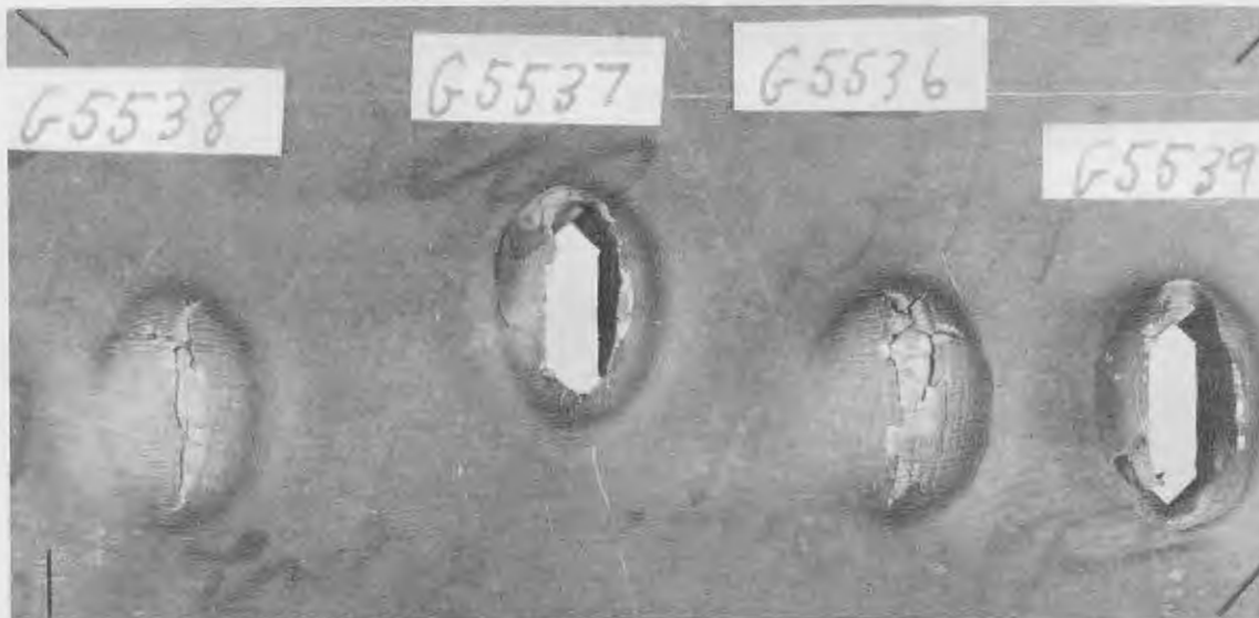
Figure 12 - Rear face damage in 3/8-inch plate of heat 2213, alloy Type IV (6 Mg/Li - 6 Al). This alloy is ballistically stronger than those shown in Figures 10 and 11 (binary Mg/Li). Note the tendency to form circumferential cracks.
