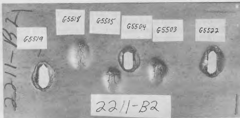
(a) Rear face 3/8-inch-plate, heat no. 2211
