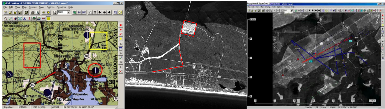
Figure 3. Examples of multi-UAV control using Falcon view. O(1) designating search area, O(n) setting waypoints, O(>n) timed rendezvous requiring multi-UV synchronization.
