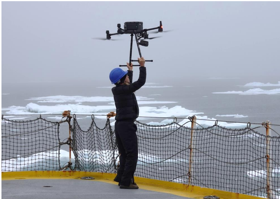
Figure 62. Hand-catch landing of the UAS assisted by the visual observer.
