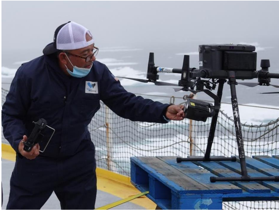
Figure 61. Pilot conducts a pre-flight visual inspection of the UAS on a wooden platform.
