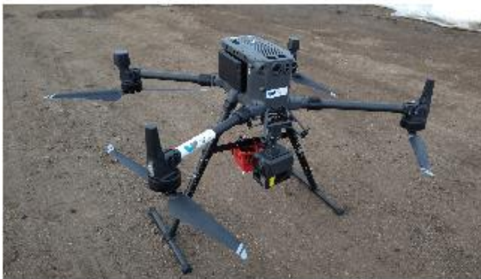
Figure 1. Left: Quadcopter with multispectral and thermal sensors. Right: Skydio X2D.
