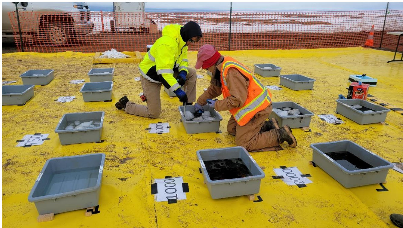
Figure 6. Totes setup in Oliktok Point, AK with different oil/ice pairings.
