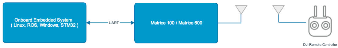
Figure 2.3. The Generic Hardware Setup for DJI's Onboard SDK. Source: [15].
