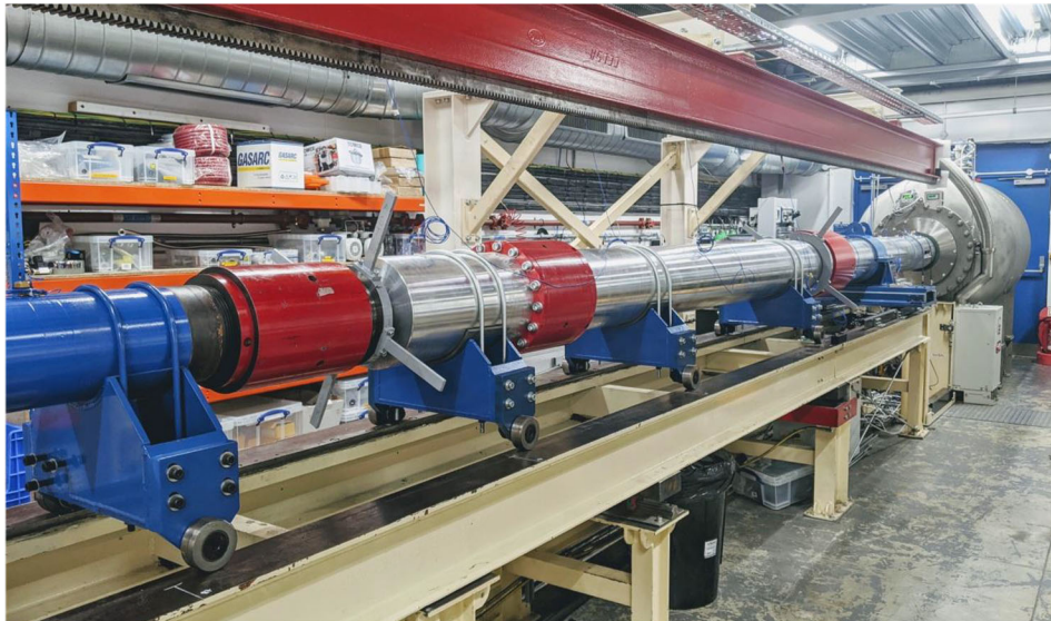
Fig. 3 The T6 Aluminium Shock Tube, connected to the secondary driver (left) and dump tank (right)
