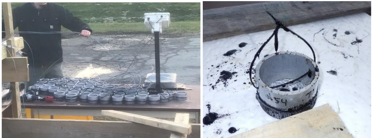
Figure 7. Sunken dilbit catchment trays.
