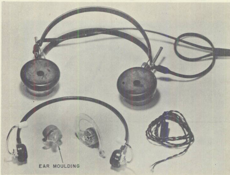
Figure 5 - Comparison of earpieces used in system compared to old type headphones
