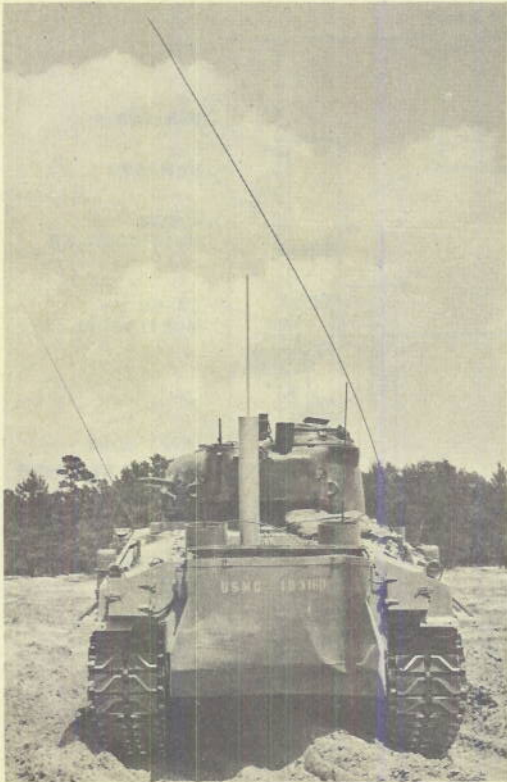
Figure 12 - Communication control tank with four-antenna installation, right side view
