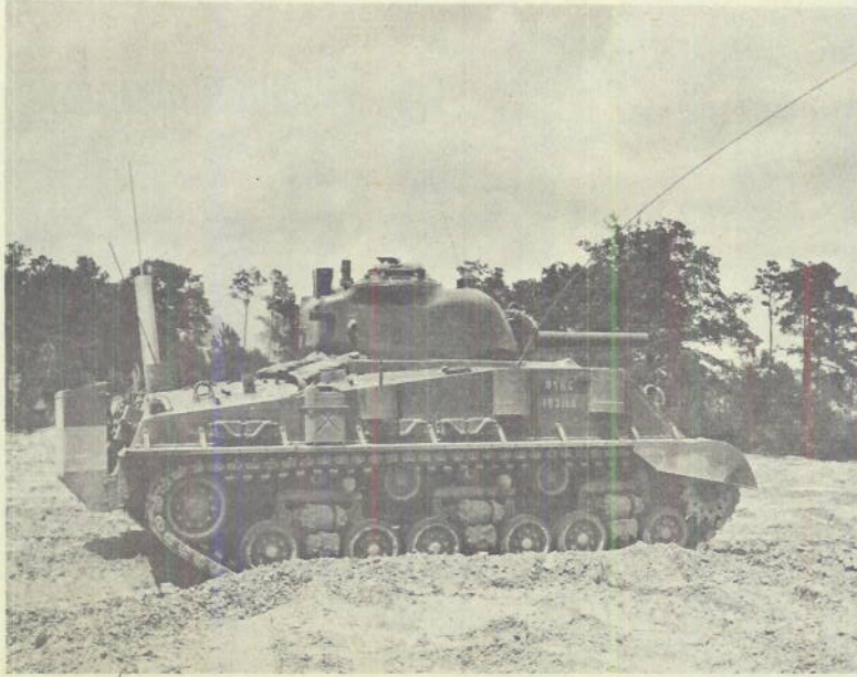
Figure 12 - Communication control tank with four-antenna installation, right side view
