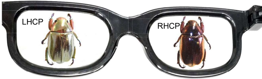
Figure 1. Left-hand circularly polarized light (LHCP) is seen through the left LHCP lens and right-hand circularly polarized light (RHCP) is seen through the right RHCP lens; because this gold beetle species strongly reflects LHCP but not RHCP, it appears different and the color is extinguished under the RHCP.
