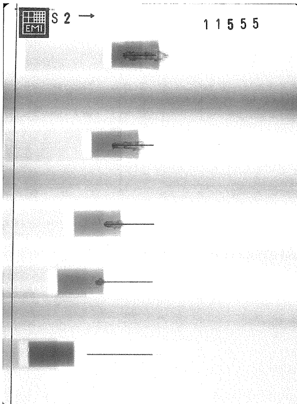
Figure A-15. X-ray picture for Exp. 11555: v_p = 2.800 km/s.
