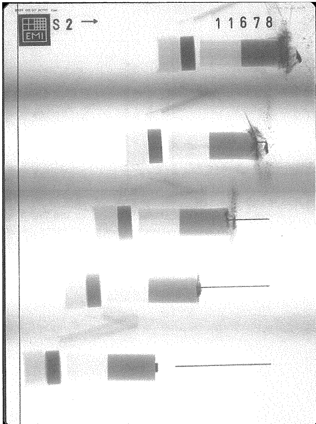
Figure B-31. X-ray picture for Exp. 11678: B2 buffer, v_p = 1.564 km/s.
