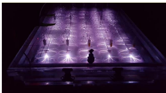
Figure 8 A Plasma reactor layout, a photo of bench scale plasma treatment unit, and a schematic of Plasma Destruction, courtesy of Clarkson University
